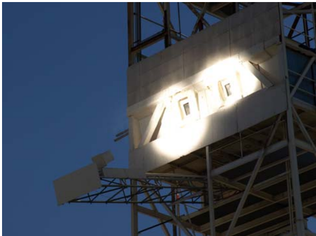
Figure 4.13. 100 kW th dual chamber pilot reactor during thermal testing at the SSPS tower at PSA.
