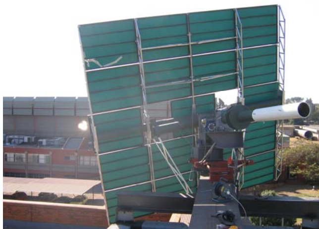
Figure 5.2 Rear view of heliostat, showing focal spot on target wall
