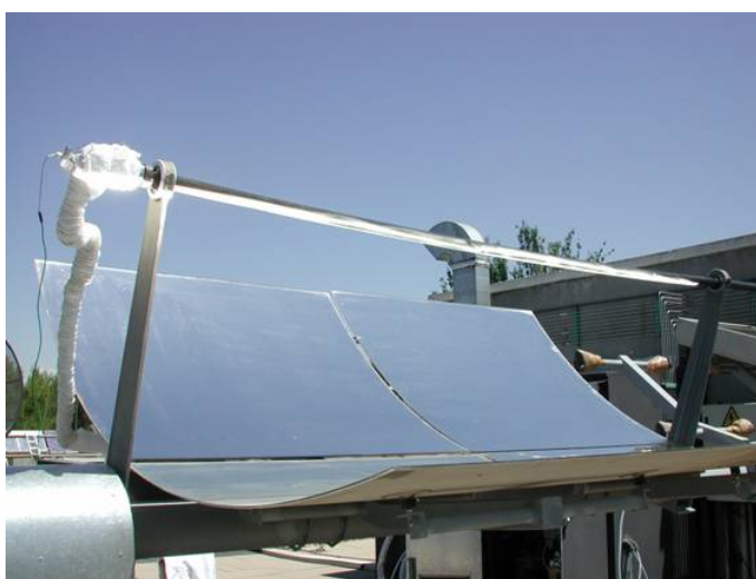
Figure 8.12 Parabolic Trough Collector used for heating air and treatment experiments.
