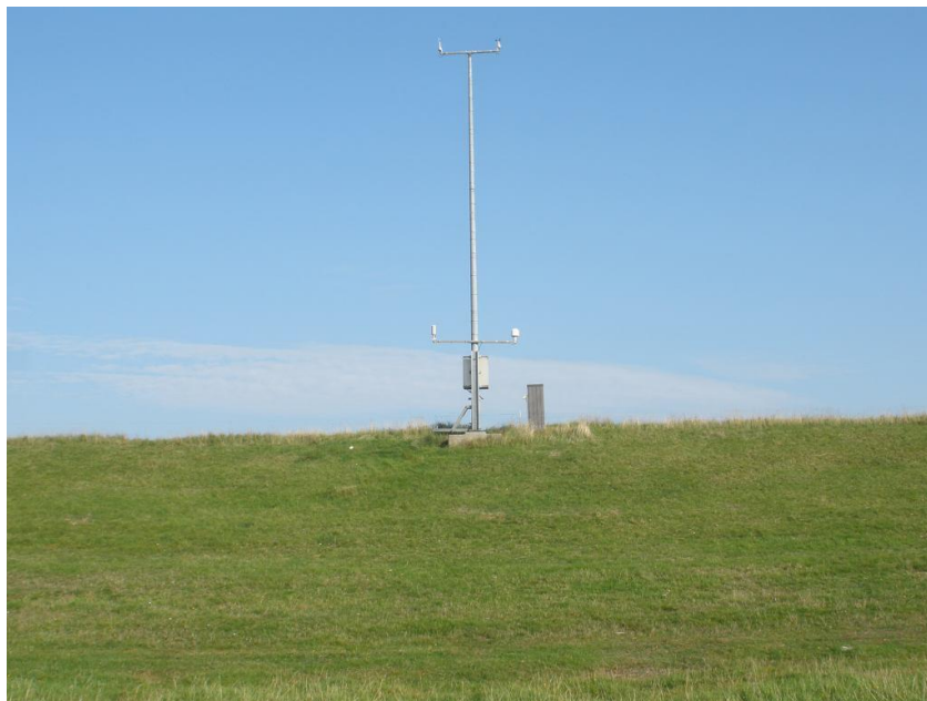
Figure 3.1. A synoptic weather station (WMO 06090). Instruments for measuring wind speed and direction are located on the 10-meter boom. Instruments for measuring temperature, humidity and global horizontal irradiance (GHI) are located on the 2-meter boom. At other stations GHI is measured on a separate post.
