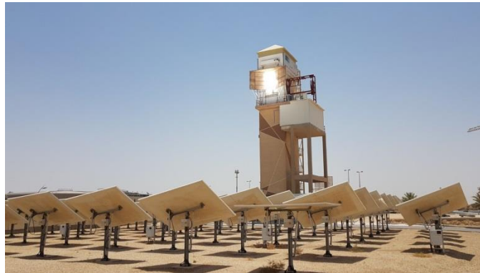
FIGURE 1. Photograph of the particle heating receiver test facility at King Saud University during an on-sun test
