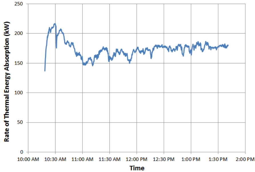
FIGURE 7. Rate of thermal energy absorption at the PHR during the test
