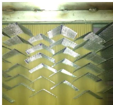
FIGURE 2. Flow of sand through a chevron particle heating receiver
