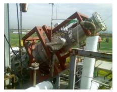
Solar steam gasification of carbonaceous feedstock
