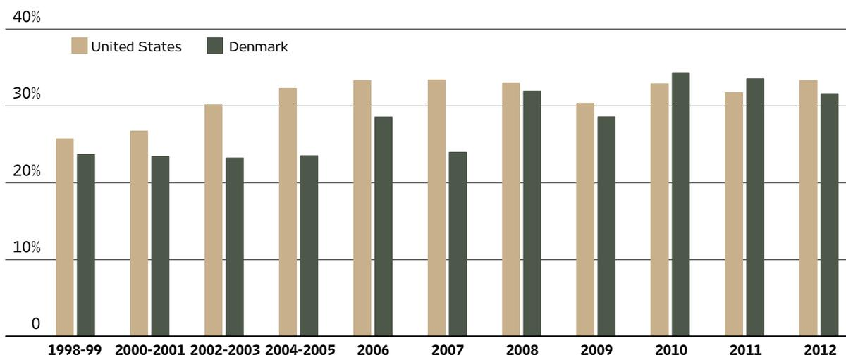
Note: Data for the United States present capacity factors in 2013 for wind turbines installed from 1989 onwards. Data for Denmark present average capacity factors for wind turbines installed from 1998 onwards.
