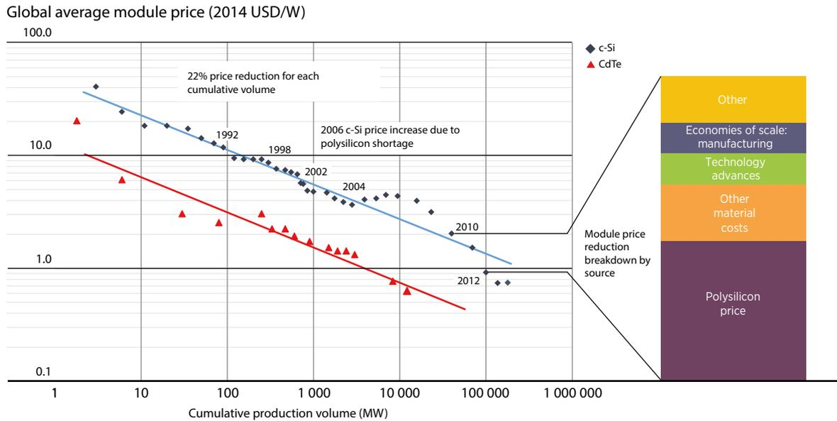
Sources: Based on data from EPIA and the Photovoltaic Technology Platform, 2011; GlobalData, 2014; GTM Research, 2014; Liebreich, 2011; pvXchange, 2014 and IRENA analysis.
