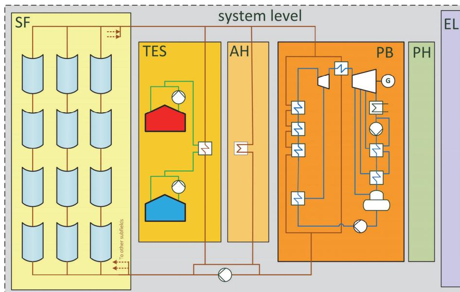
Figure 3-1: Break-down into sub-systems for the example of a parabolic trough oil system
