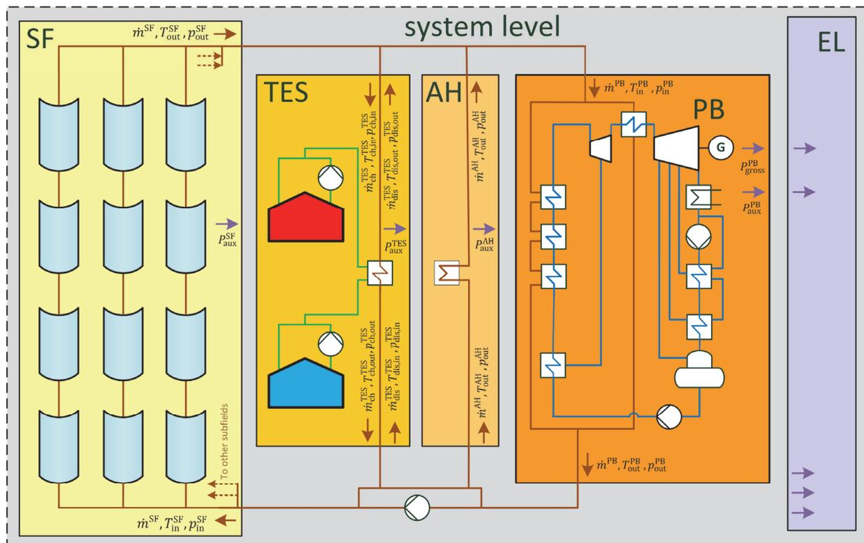
Figure 4-1: Sub-system schematic with main interface variables for a parabolic trough plant with two-tank storage and auxiliary heater
