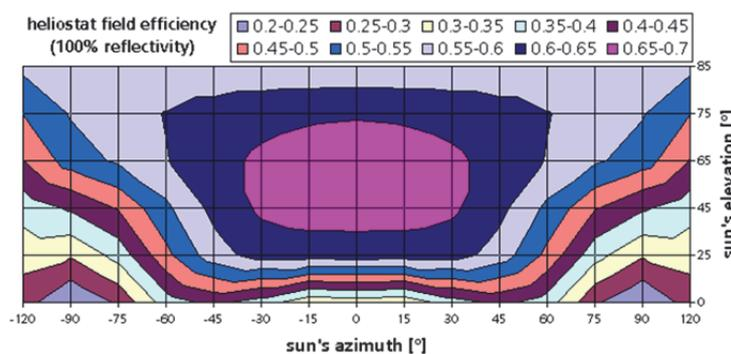
Figure 5-8: Illustration of optical losses in the heliostat field in terms of  $\eta_{\text{conc,opt}^*}(\alpha_s, \gamma_s)$
