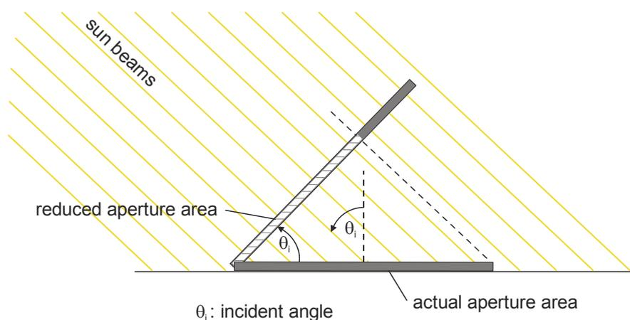
Figure 5-3: Effective aperture reduction caused by non-perpendicular sun rays onto the aperture (cosine losses)
