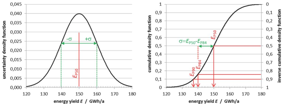
Figure 13-1: Uncertainty density distribution (left) and cumulative density function (right) of the energy yield
