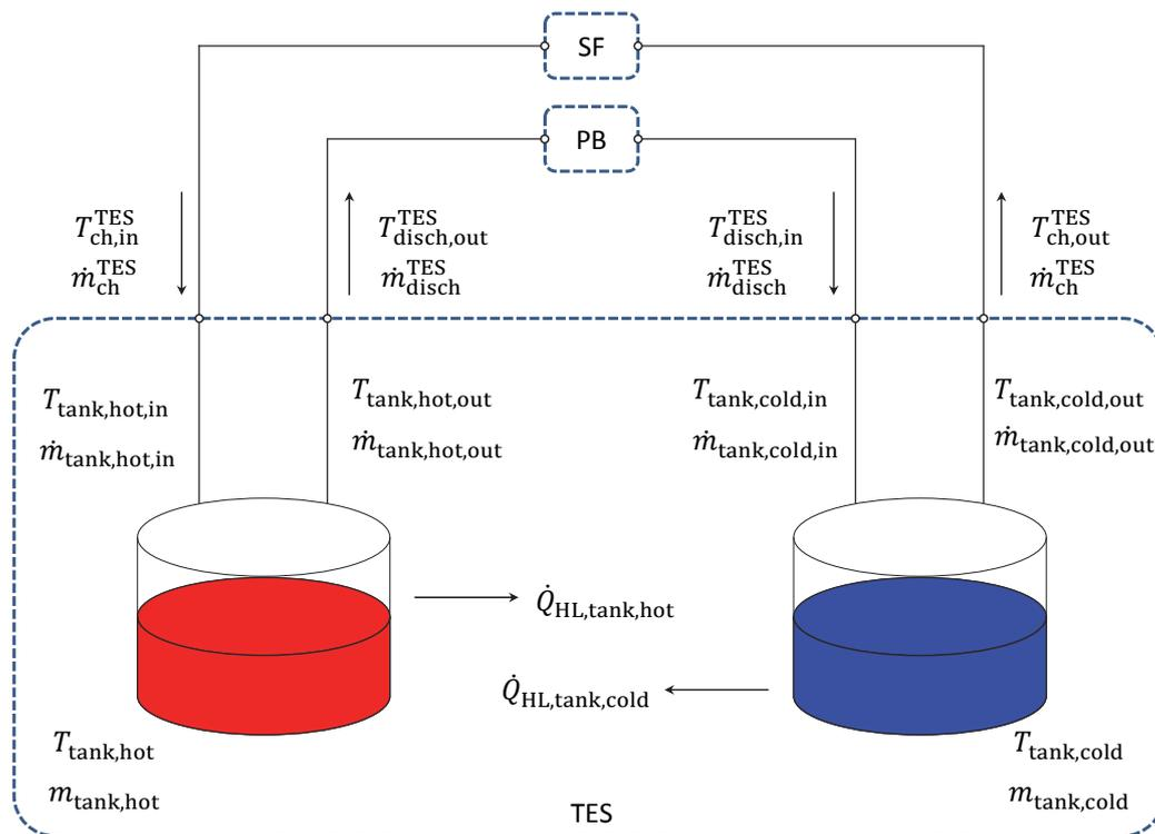
Figure 7-2 Scheme of a two-tank direct molten salt storage system
