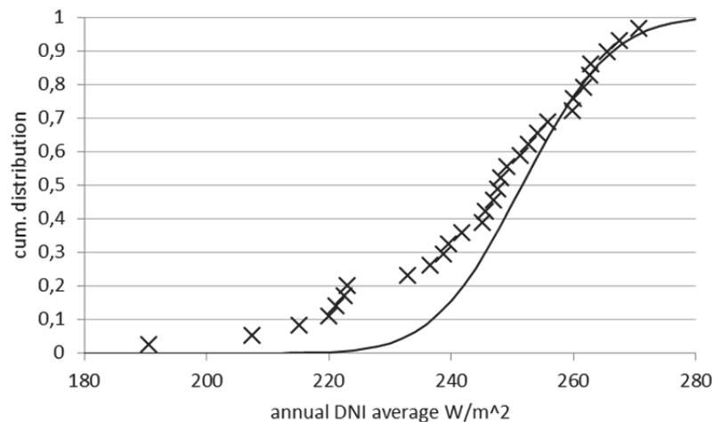
Figure 12-2: Cumulative distribution function of the time series given in Figure 12-1 (crosses) and the corresponding normal distribution based on the mean ( $251,2 \text{ W/m}^2$ ) and standard deviation ( $s=12 \text{ W/m}^2$ ) of the time series
