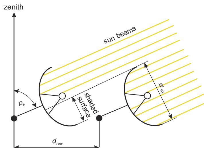
Figure 5-4: Row-to-row shading in a parabolic trough solar field
