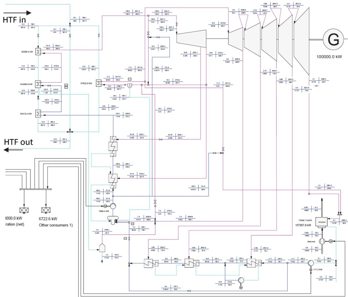
Figure 6-2: Heat flow diagram for a Rankine cycle with re-heater operated with thermal oil
