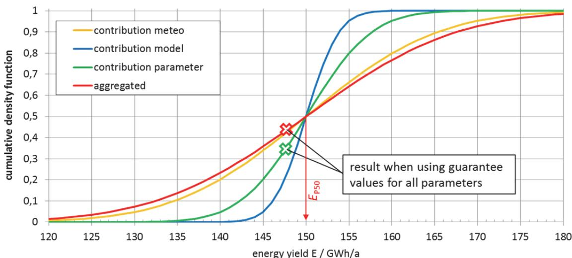
Figure 13-7: Result of the probabilistic analysis for model parameters with marked values for mean and guarantee value.
