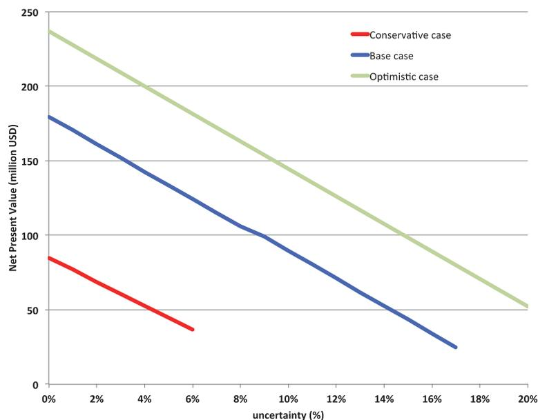
Figure 2-3 Impact of energy yield uncertainty and financing conditions on the net present value (lines terminate when DSCR falls below the threshold or the setup would not allow a project finance any more)
