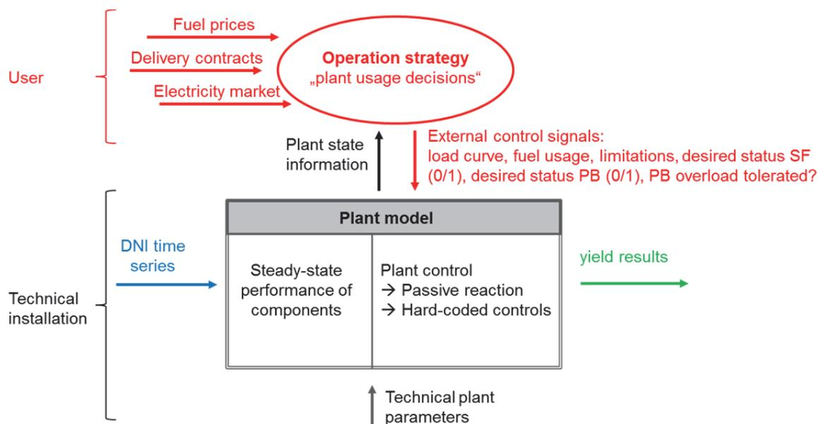
Figure 10-2: Interface between plant control and operation strategy
