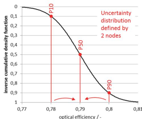
Figure 13-6: Distribution function reflecting the impact of guarantee values for the example of the optical efficiency
