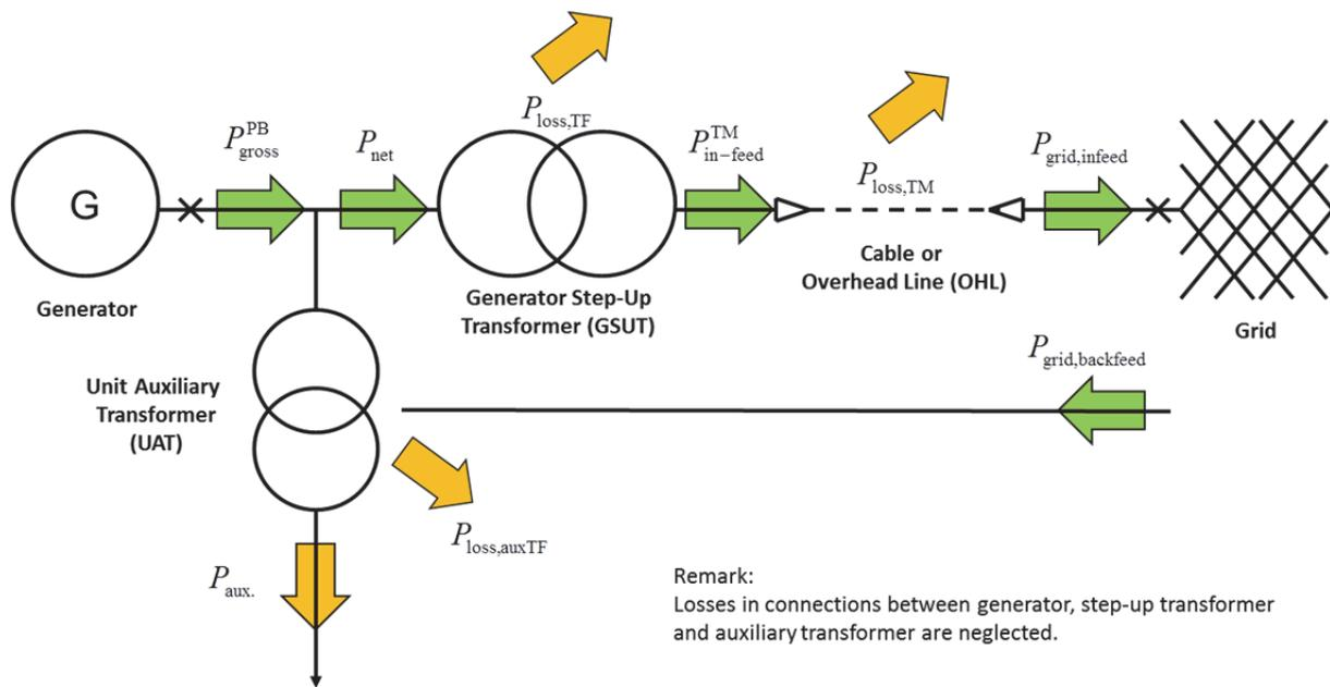
Figure 9-1: Simplified single line diagram and losses of electrical system for normal operation
