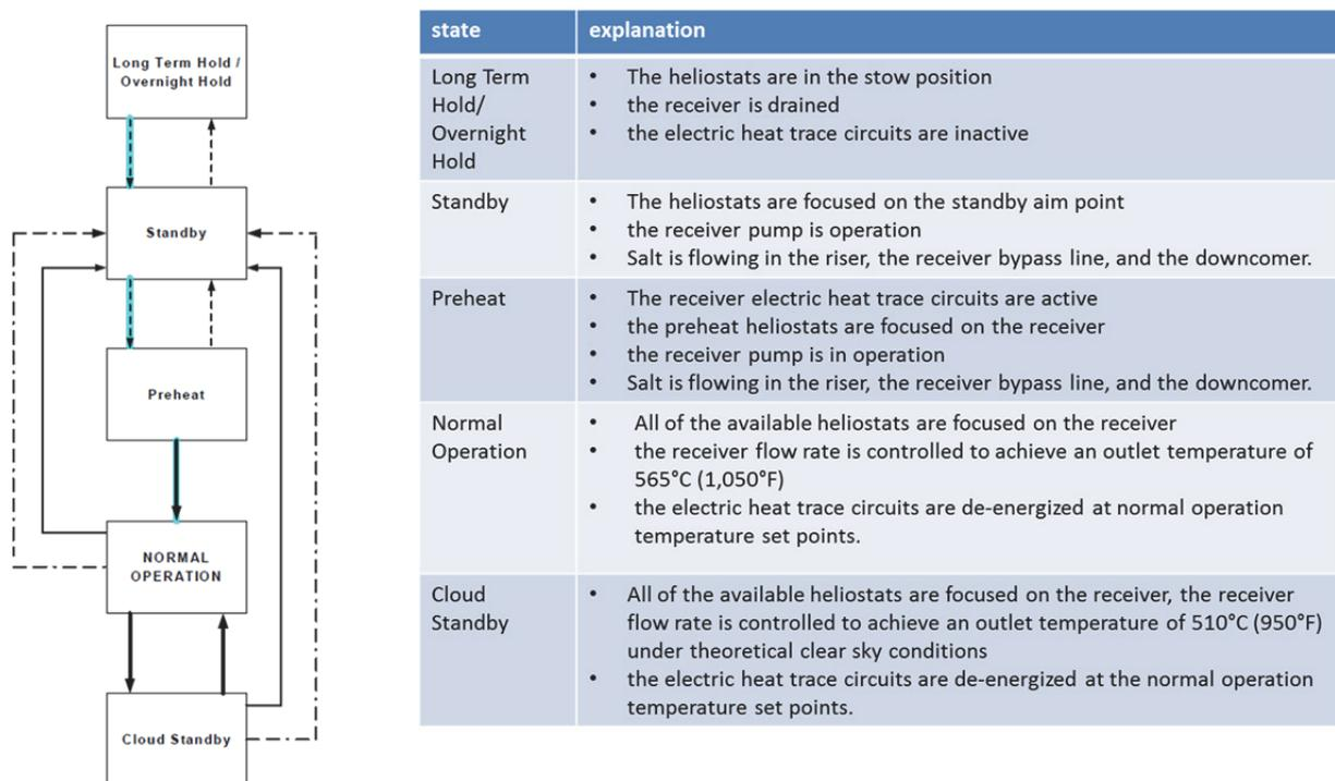
Figure 5-10: Operation states of a receiver system of a molten salt tower<sup>18</sup>
