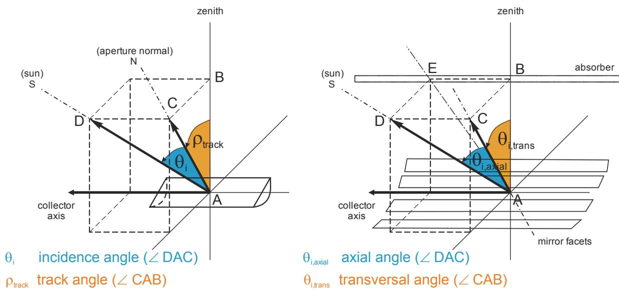
Figure 5-2: Angle definitions for parabolic troughs (left) and linear Fresnel collectors (right)
