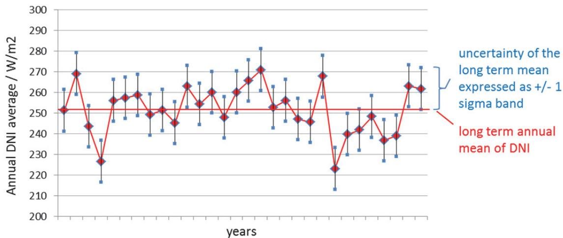
Figure 12-1: Illustration of DNI long-term mean ( $251,2 \text{ W/m}^2$ ), its uncertainty of the long-term mean ( $10 \text{ W/m}^2=4\%$ ), and inter-annual variability ( $s=12 \text{ W/m}^2$ )
