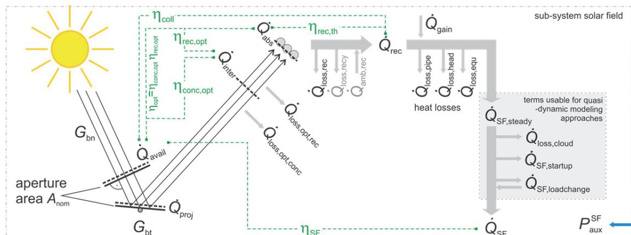
Figure 5-1: Illustration of generic variables for the sub-system solar field (please note that not all technologies require all of these variables)
