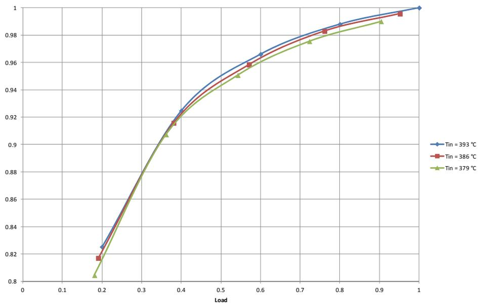
Figure 6-4: Impact of load,  $\dot{Q}^{PB} / \dot{Q}_0^{PB}$ , and inlet temperature,  $T_{in}^{PB}$ , on the gross efficiency correction function  $f_1$  for a thermal oil driven Rankine cycle with wet cooling tower.
