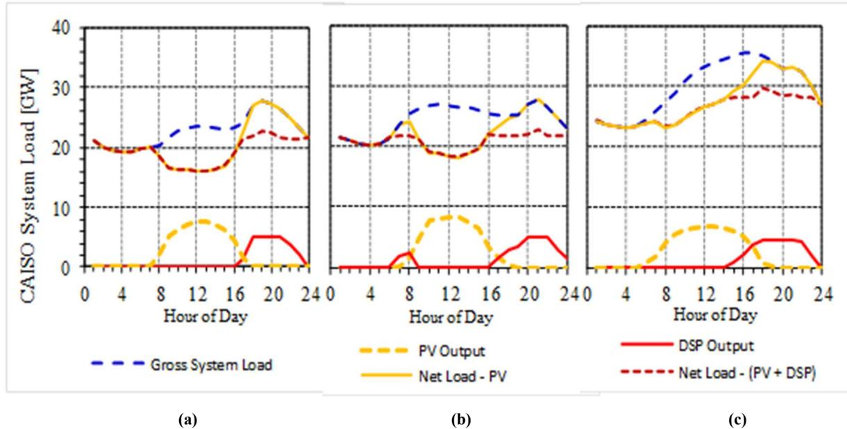
FIGURE 2. Example of a MS Tower DSP Plant in Operation: (a) Winter, (b) Spring, (c) Summer
