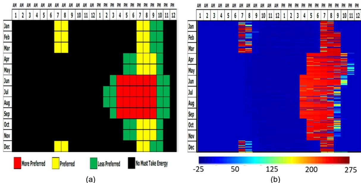
**FIGURE 4 Sample DSP Plant Application: (a) APS 2017 Peaking Capacity RFP Time of Delivery Periods, (b) SAM Optimized DSP Dispatch Model for Nominal 400 MWt Solar Field (TMY Case)**
