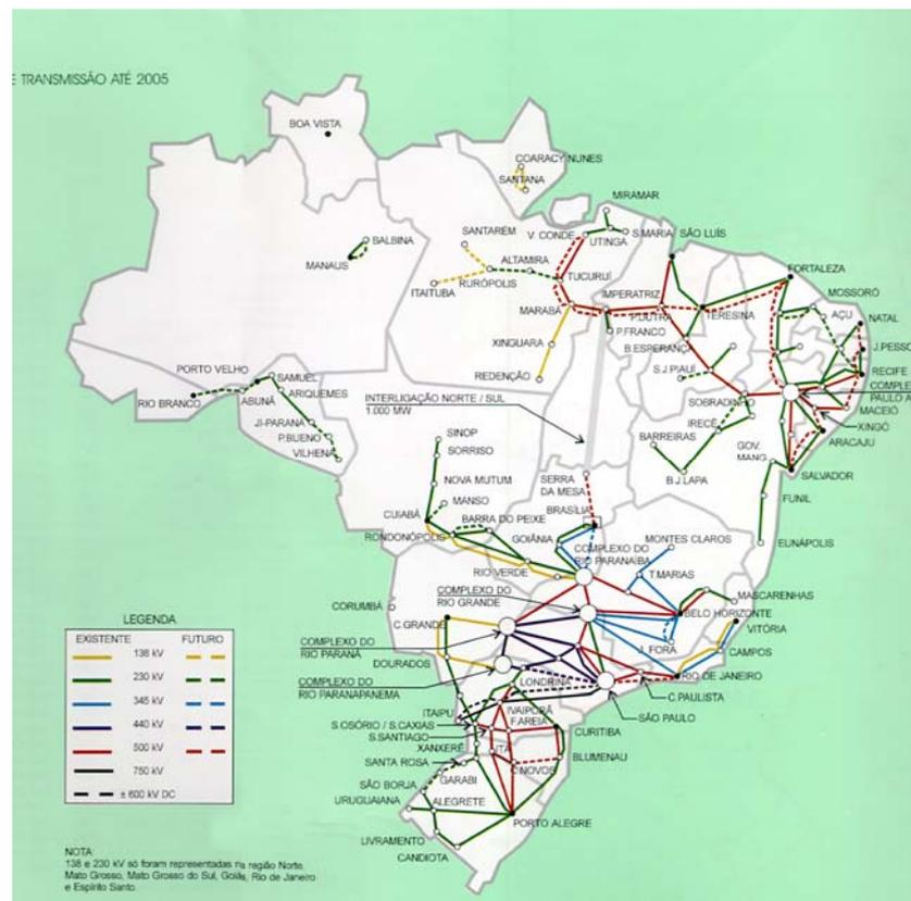
Figure 5.13 Map of transmission lines (Source ELETROBRÁS Relatório Anual 1995)
