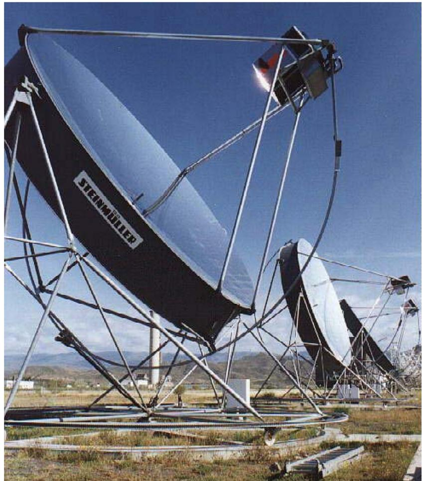
Figure 3.10 New SBP 10kW Dish-Stirling System at the Plataforma Solar de Almería, Spain
