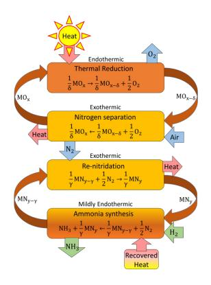
The STAP process consists of two cycles. The first cycle (top) illustrates nitrogen separation from air using concentrated solar heat. The second cycle (bottom) ammonia production at pressure an order of magnitude lower than HB.
