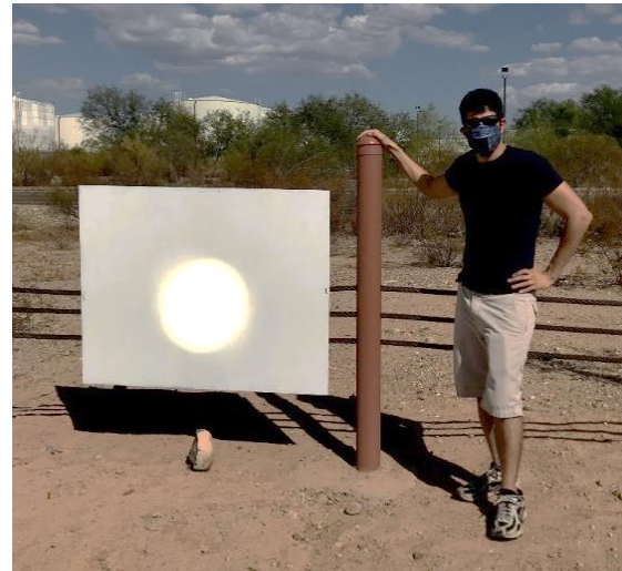
FIGURE 3. (a) surface measurement of the reflector shape actuated for 62^\circ AOI from its base shape for 45^\circ AOI and 40 m focal length (b) image of the solar disc at 62^\circ AOI.
