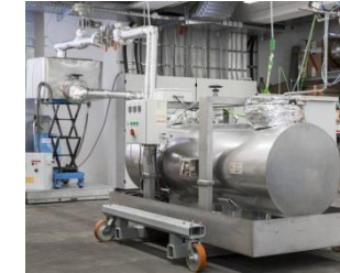
Molten salt loop for gravimetric calibration of flow meters at FRAUNHOFER ISE
