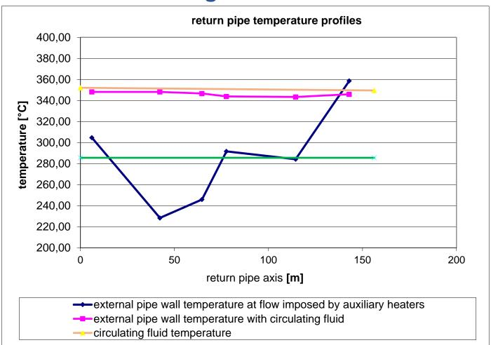
Wall temperature profile vs the axis of the return pipe in conditions of imposed temperature (circulating fluid) and imposed flow (non-circulating fluid, heating with heating cables)
