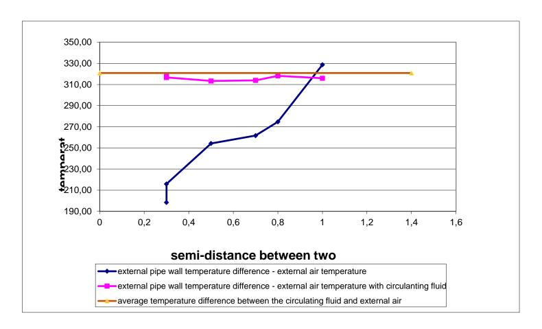
Wall temperature profile vs half of the distance between the poles of two consecutive supports (constraints) of the return pipe in conditions of imposed temperature (circulating fluid) and imposed flow (non-circulating fluid, heating with heating cables).
