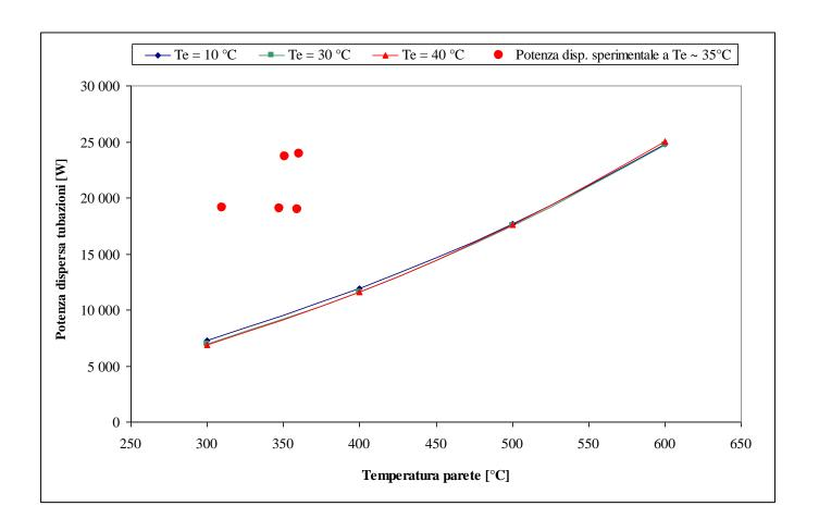
Thermal power dispersed by the return pipe and the average wall temperature. Calculated values compared with experimental ones, in conditions of imposed temperature (circulating fluid).
