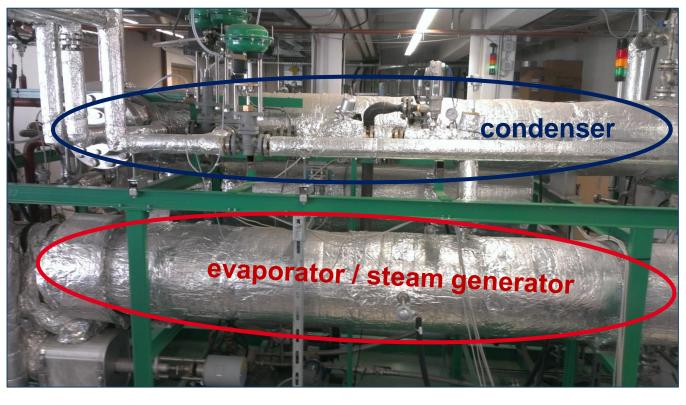
The steam facility at ISE's high-temperature lab mainly consists of:
