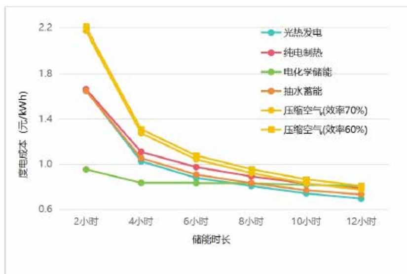
Fig. 6.2-3: LCOE (per kWh) of CSP + MS TES and PV + different energy storage systems
