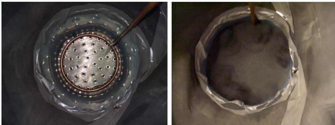
Fig. 112: “Annular” fluidized bed trials. Left: Provisional gas distributor made of a copper ring. Right: Annular bubbles distribution on the surface of the fluidized bed.
