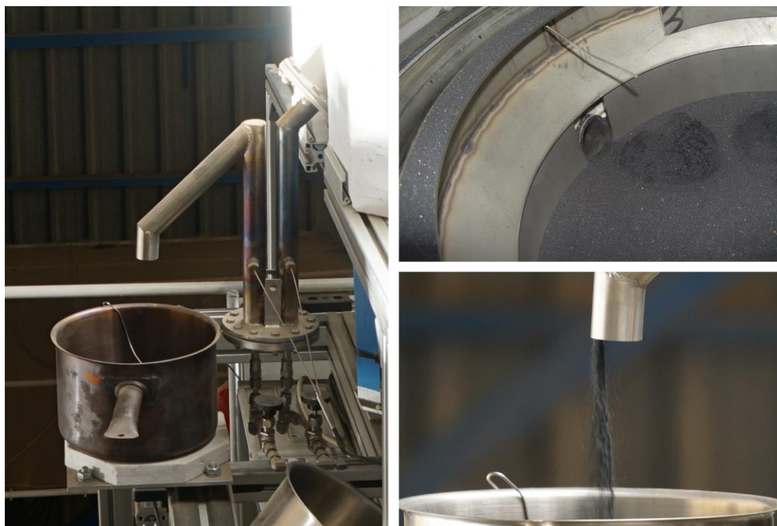
Fig. 67: Particle removal from the reactor. Left: Siphon shaped Outpipe. Right top: Overflow inside the reactor. Right bottom: Solids outflow.
