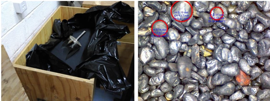
Fig. 48: Kenmare Moma Ilmenite, grain size 150 µm. Left: In the storage box. Right: Magnified.
