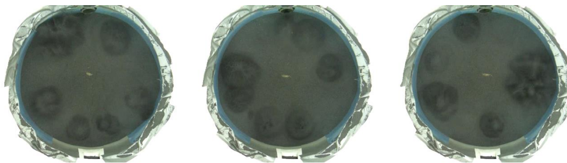
Fig. 115: Bubbling of the fluidized bed with “annular” fluidization
