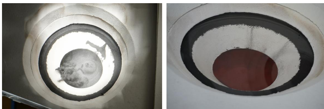
Fig. 126: Left: Well fluidized particles. Right: Red hot glowing particles at 800 °C.
