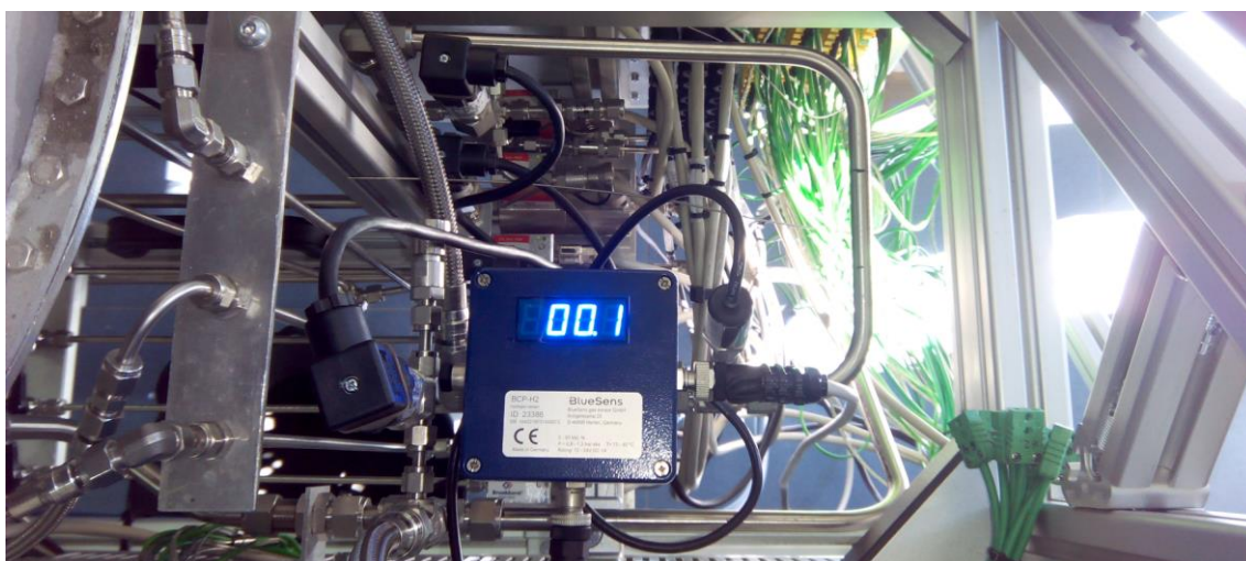
Fig. 94: Hydrogen sensor in the reactor feed gas line.
