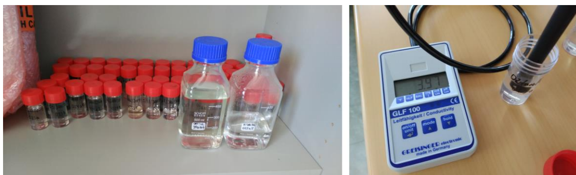
Fig. 148: Left: Product water samples from the Oresol tests. Right: Conductivity measurement.
