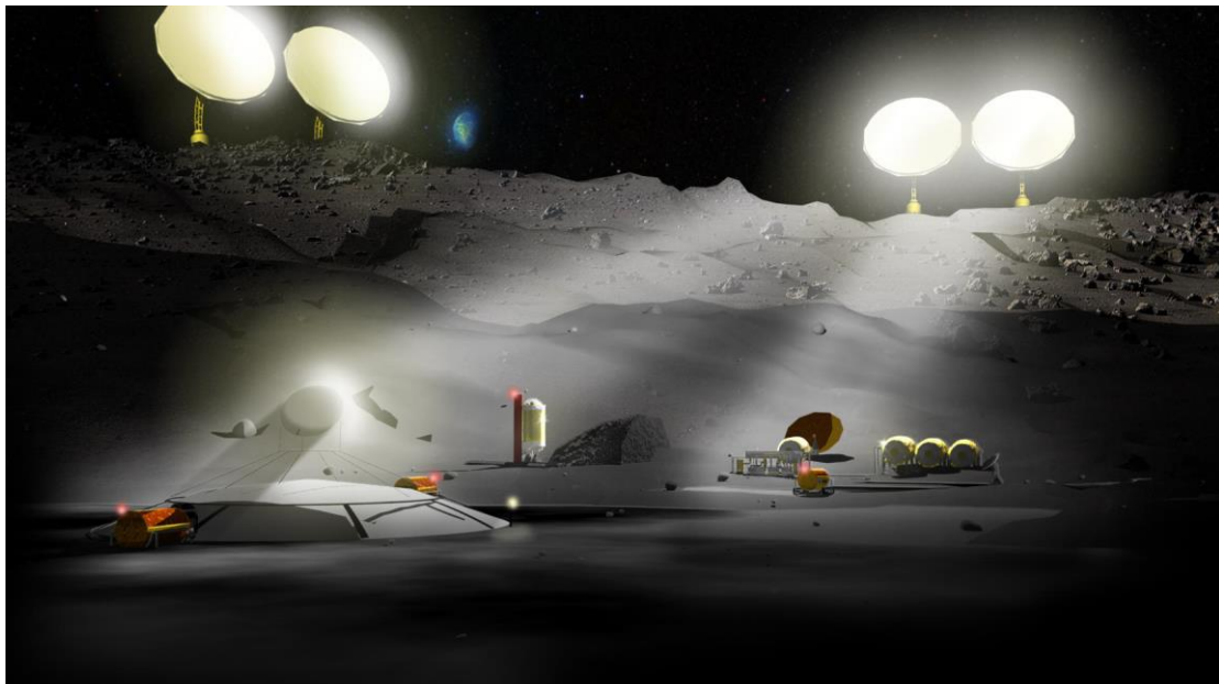
Fig. 15: Lunar polar ice mining with direct solar power supply from large heliostats located on the rim of the crater. From (Sowers, 2020).
