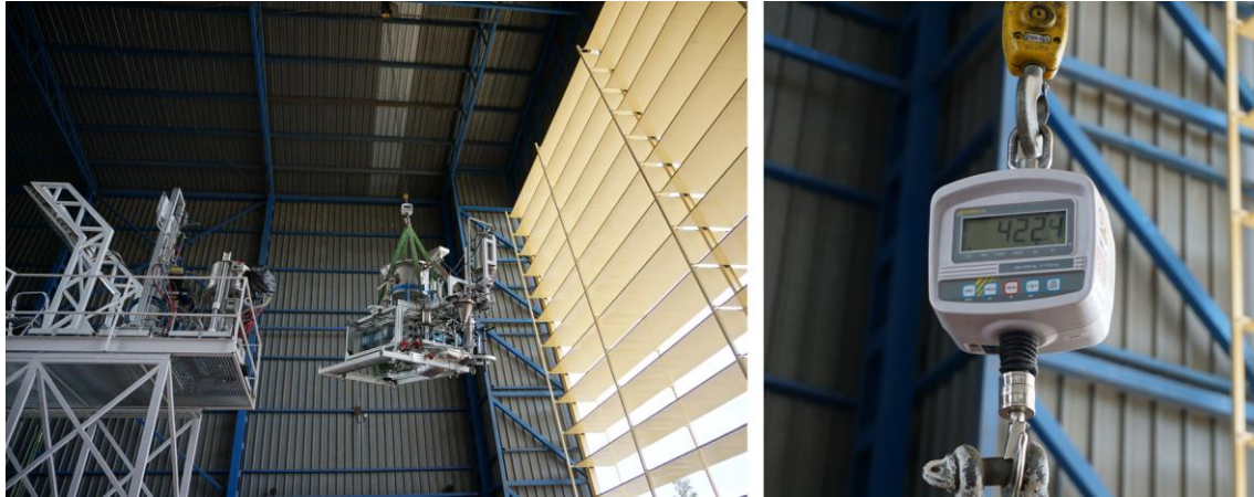
Fig. 123: Lifting of the Oresol plant onto the test platform of the Solar Furnace SF-60 for the second test campaign.
