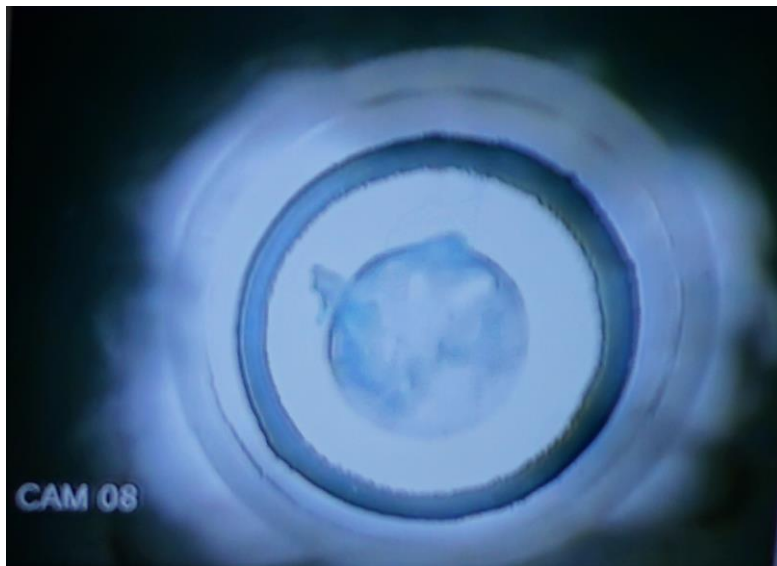
Fig. 139: Monitor for observation of the fluidized bed during operation.
