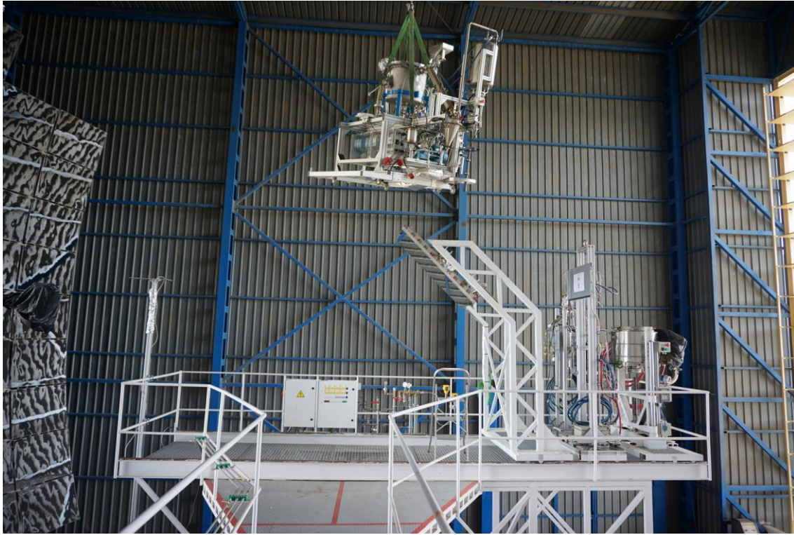
Fig. 91: Lifting of the entire Oresol experiment onto the test platform of the Solar Furnace
