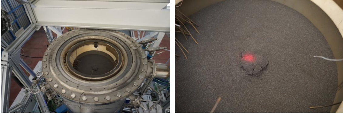
Fig. 122: Slightly sintered material in the center of the reactor (the red dot is from a laser for calibration).
