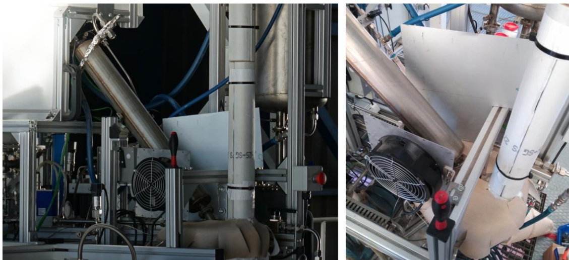
Fig. 131: Cooler C1 converted into an air cooler with fan.
