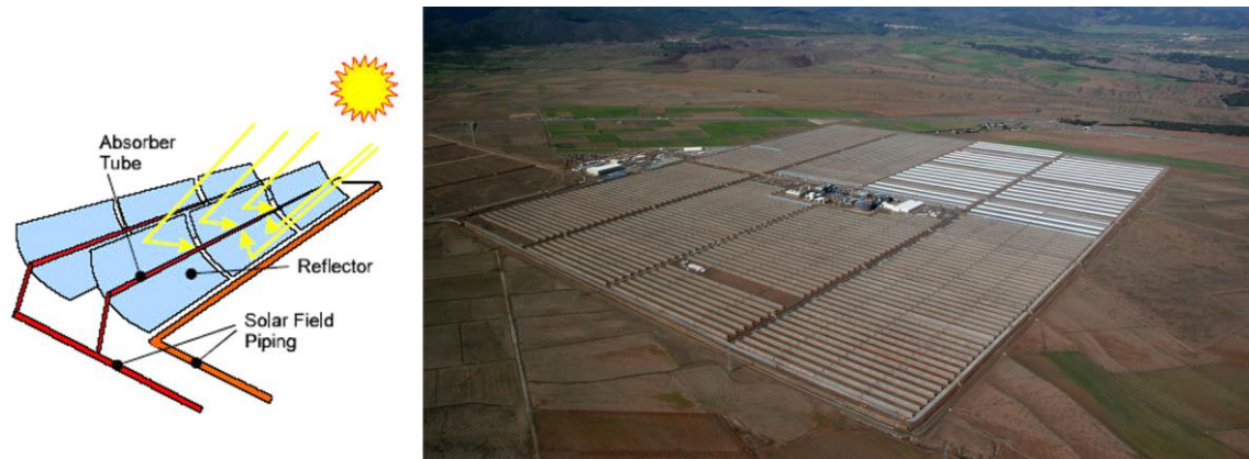
Fig. 21: Parabolic trough (line concentrating) systems. Left: Operational principle (SolarPACES, 2018). Right: Aerial view of the Andasol plant in southern Spain 36 .
