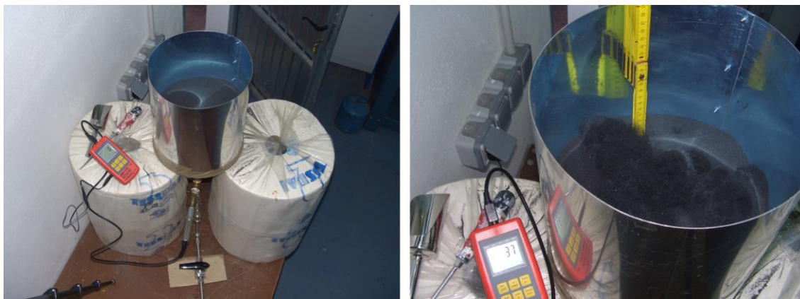
Fig. 110: Very first fluidization test with Ilmenite-150. The 40-screws gas distributor “40/3” (see chapter 3.5.4) was used. The red instrument is a handheld display for pressure sensors that later could be attached with quick connectors to various points of the system.
