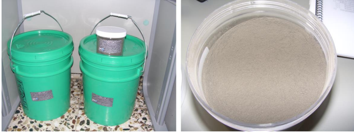
Fig. 47: JSC-1A Lunar Soil Simulant.
