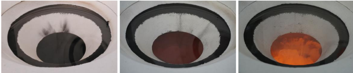
Fig. 17: Photographs of the Oresol reactor at 400 °C (left), 800 °C (center), and 950 °C (right). The color and brightness difference of the emitted radiation due to the different temperatures is clearly visible.
