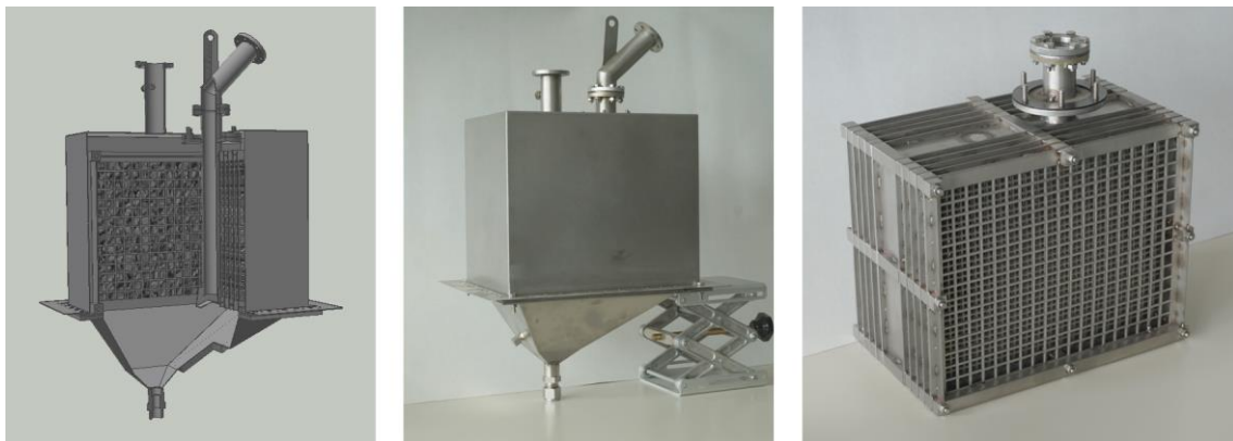
Fig. 154: New off-gas filter with 20x increased filter area.
