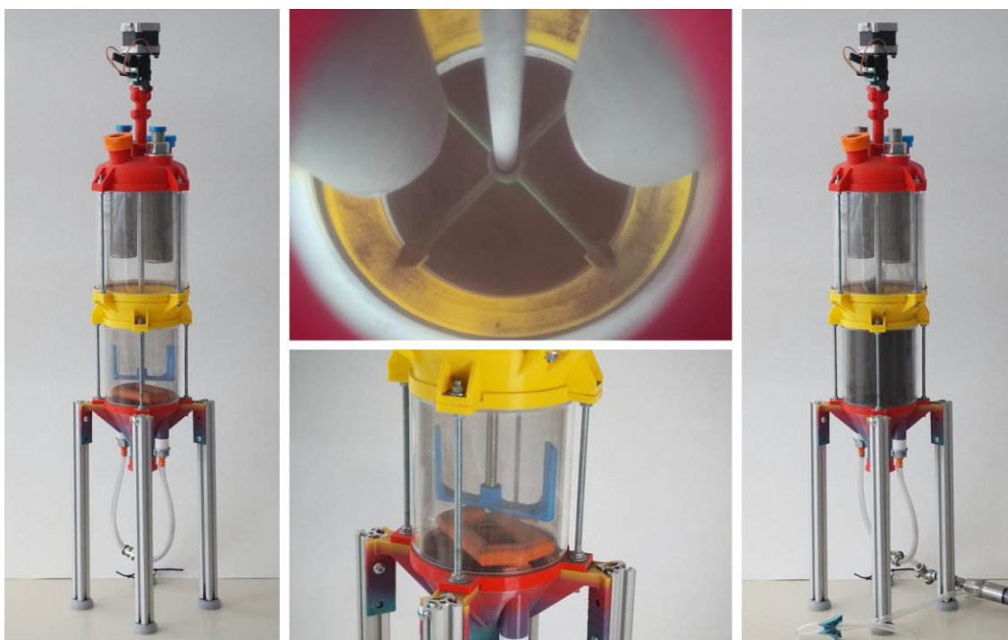
Fig. 11: 3D-printed cold model for demonstration purposes of the ALCHEMIST reactor. Left: Empty “reactor”. Right: Filled with particles. Top: Look into the viewport; the two filter candles, the shaft of the stirrer, and the surface of the fluidized bed are visible. Bottom: Close-up view of the gas distributor (orange) and the stirrer (blue). The stirrer is designed to efficiently scrape the walls of the reactor, the location that is most prone for sintering.
