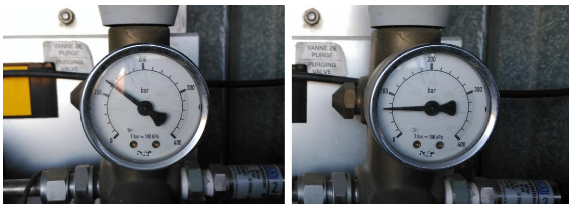
Fig. 151: Argon pressure in the bottle before (left) and after (right) the test from Jan09, 2019. The difference of 50 bar indicates that ¼ of the capacity of the bottle (10.6 m 3 ) was consumed.
