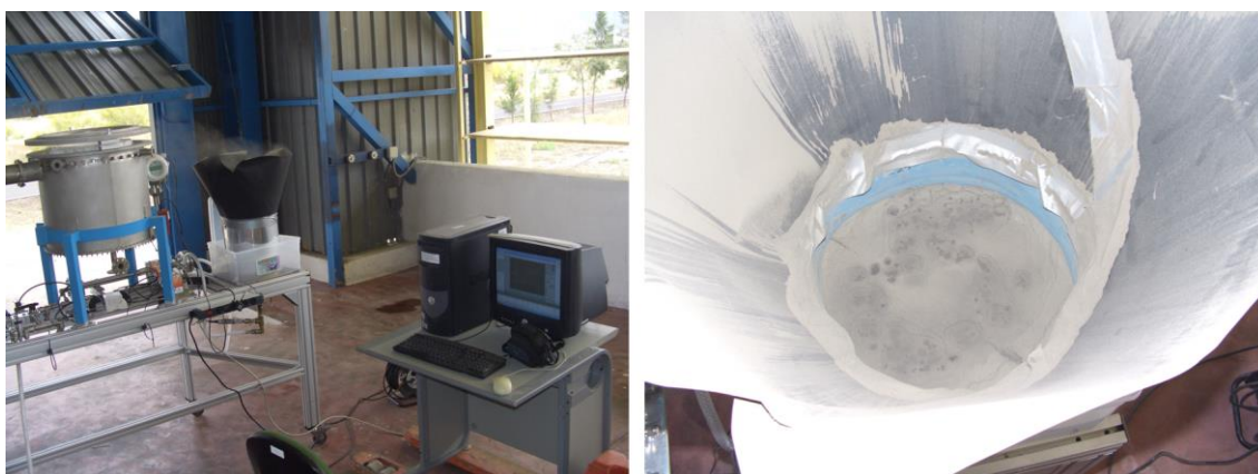
Fig. 111: Fluidization test with JSC-1A. Left: System setup. Right: View into the fluidized bed.
