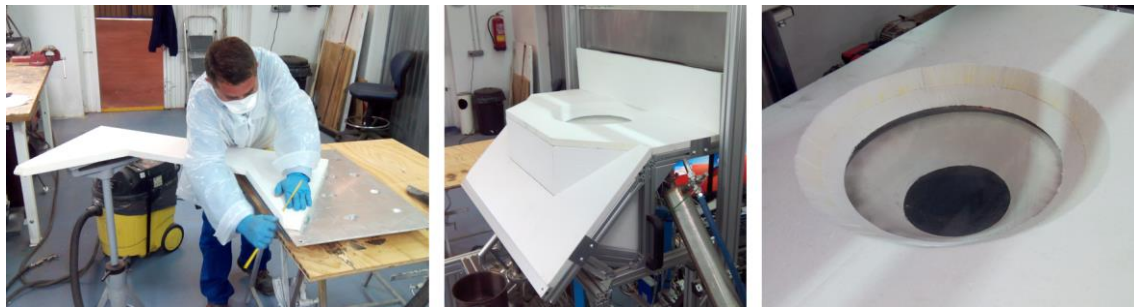
Fig. 61: Radiation shield hardware. Left: Manufacturing at the PSA Solar Furnace workshop. Center: Initial version still with the diagonal shield. Right: Conical central opening, adapted to the shape of the concentrated solar ray.
