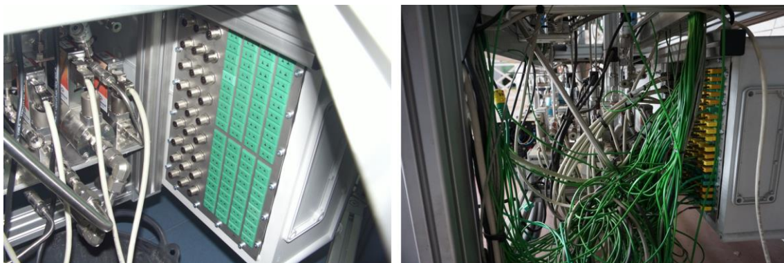
Fig. 92: Sockets for 80 thermocouples and 27 analog sensors on the backside of the electrical cabinet.
