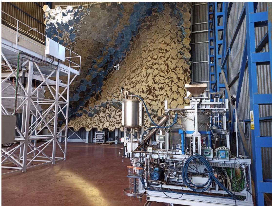
Fig. 133: Oresol system in summer 2021 awaiting future testing. In the background the recently replaced, brand-new concentrator of the PSA Solar Furnace.
