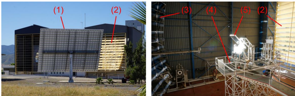
Fig. 49: Solar Furnace SF-60 of the Plataforma Solar de Almería. Left: View from outside. Right: View from inside. (1) Heliostat. (2) Shutter. (3) Concentrator. (4) Test platform with Oresol reactor. (5) Diagonal mirror. For a schematic view see Fig. 25 left on page 48.
