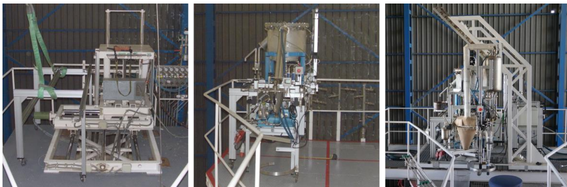
Fig. 89: Evolution of the test platform. Left: Original state with the old 3-axes table (Feb 2011). Center: Flat surface still with the steel sheet floor but the table dismantled (May 2015). Right: Current state with robust precision rails (March 2017).
