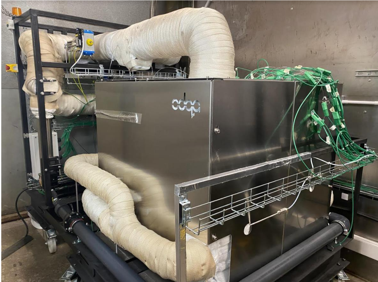
Figure 7: TES under validation at ODQA's facility
