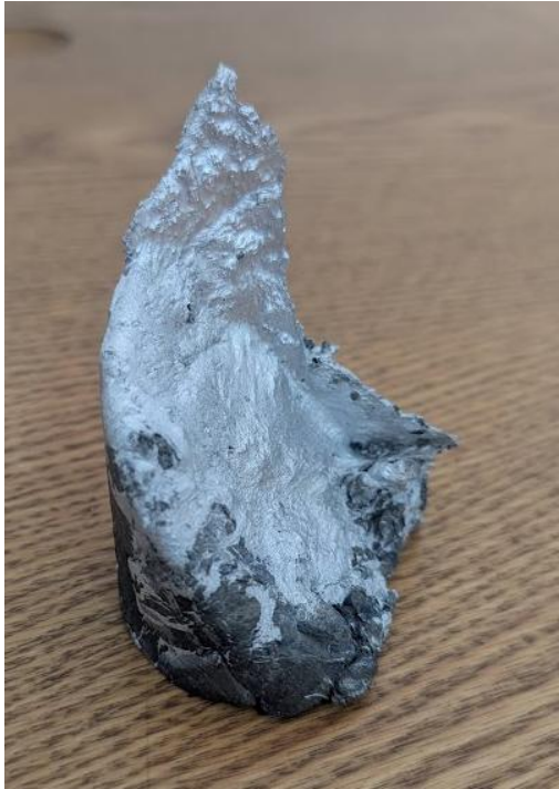
Figure 21: Picture Solidified Sample — Impurity Evidence
