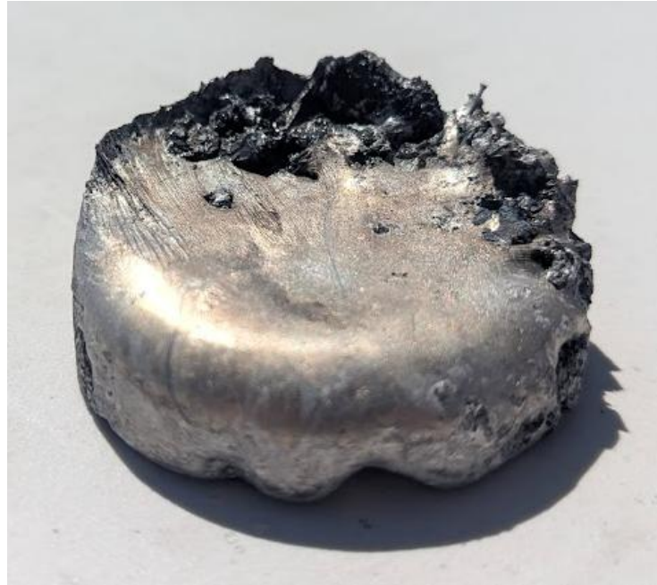
Figure 23: Cast puck — surface impurities
