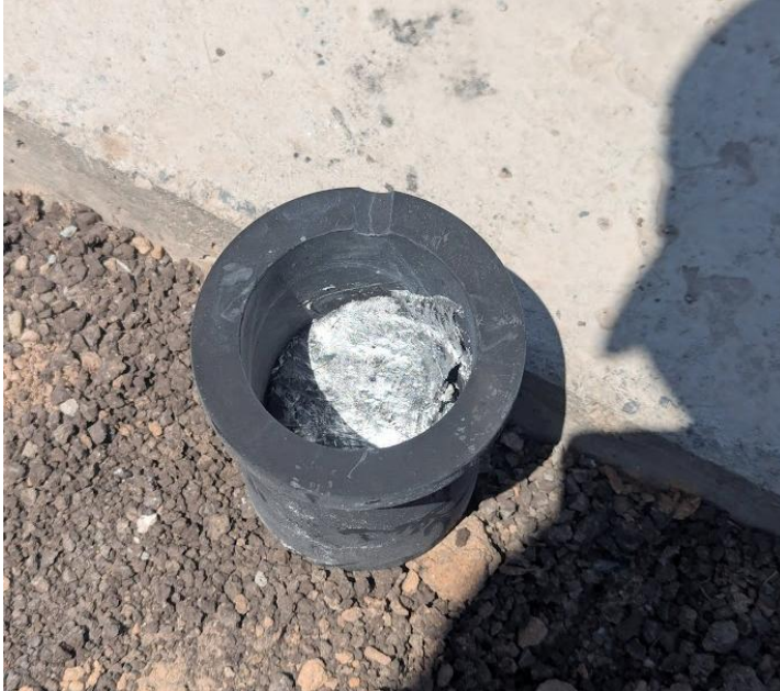
Figure 20: Picture Resulting Puck — Impurity Evidence
