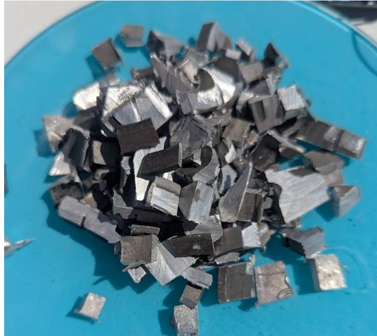
Figure 22: Feedstock — aluminum scrap (3rd test)
