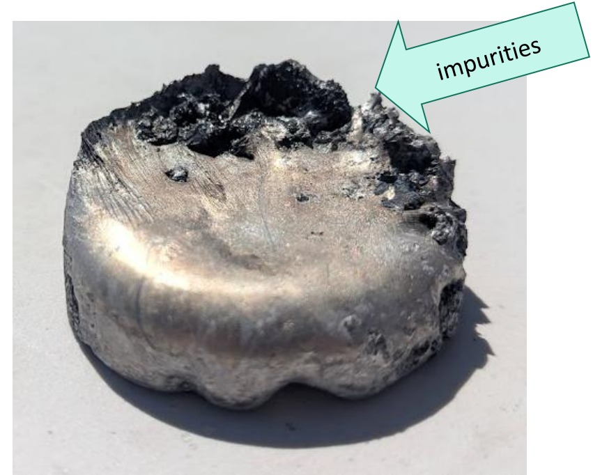
Figure 23: Cast puck — surface impurities
