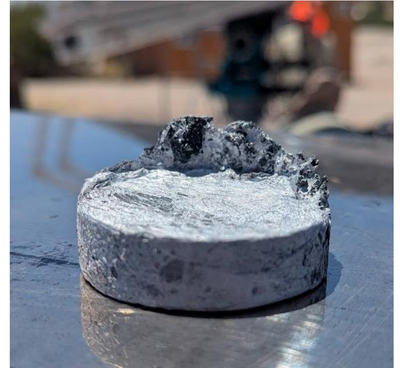
Figure 24: Cast puck — surface impurities
