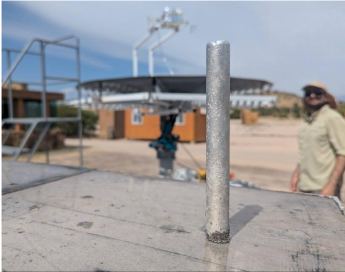
Figure 28: More pictures of remelting samples. Long tensile specimen.
