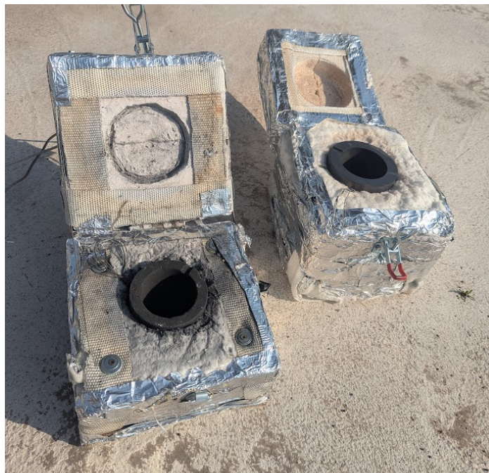
Figure 5. Images of the two custom-made furnaces manufactured for the Renoval solar furnace
