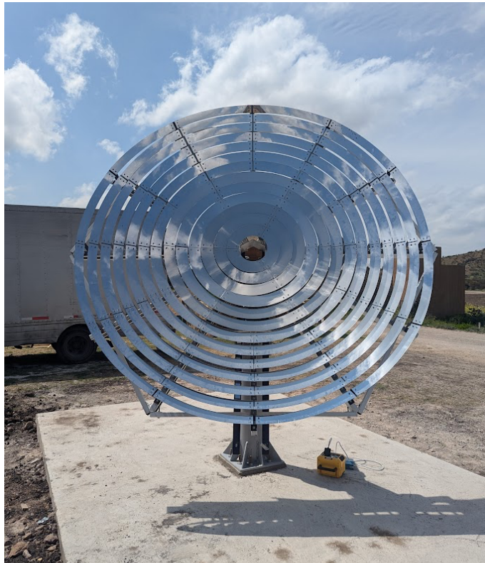
Figure 3. Image of annular Fresnel reflector installed on site.
