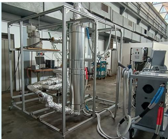
Ates Facility during thermal characterization of thermal-electrical energy storage
