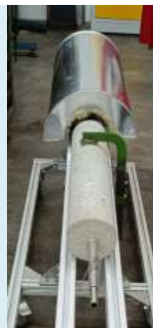
Thermal electrical energy storage module prototype using concrete with PCM encapsulated.
