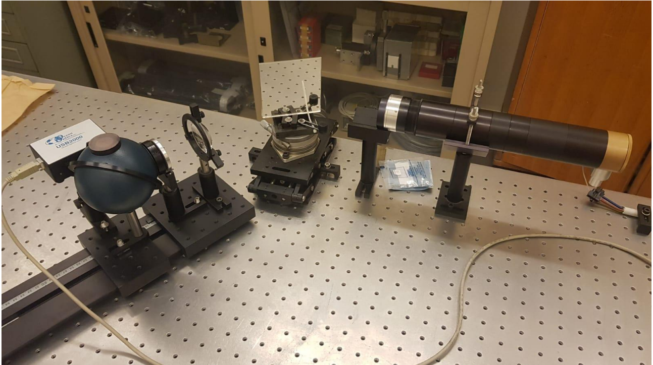
Fig. 4: SSUp configured for measurements at 60^\circ of incidence.
