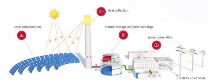
Figure: molten salt solar tower plant diagram
