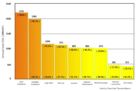
Figure: Efficiency and energy loss of a typical CSP plant
