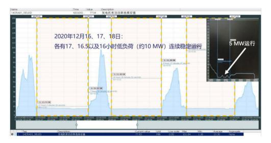
Figure: The minimum load of the steam turbine can reach 5 MW (20%~ 40% of the conventional thermal power), and help peakshaving with the stable operation in low load runs
