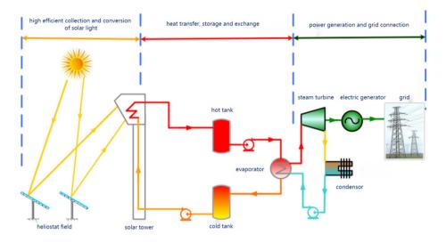
Figure: Schematic of solar tower plant with molten salt as heat transfer fluid
