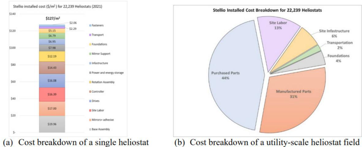
Figure: sbp Stello heliostat cost breakdown (Source: Roadmap to Advance Heliostat Technologies for Concentrating Solar-Thermal Power, 2022 Heliocon)
