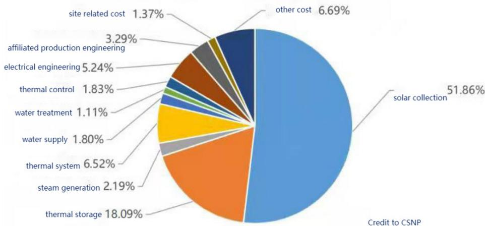
Figure: Investment composition of one 100MW parabolic trough power plant with 10h thermal storage system
