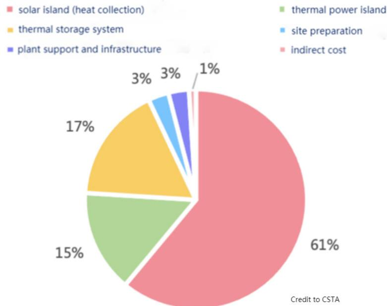
Figure: Investment composition of 50MW solar tower power plant with 7-hour thermal storage
