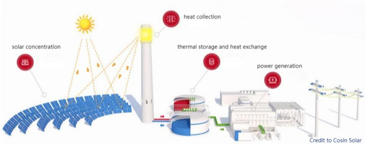
Figure: molten salt solar tower plant diagram
