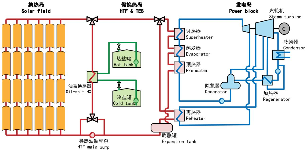
Diagram of a parabolic trough CSP plant (with conventional processes) (source: ROYAL TECH CSP )
