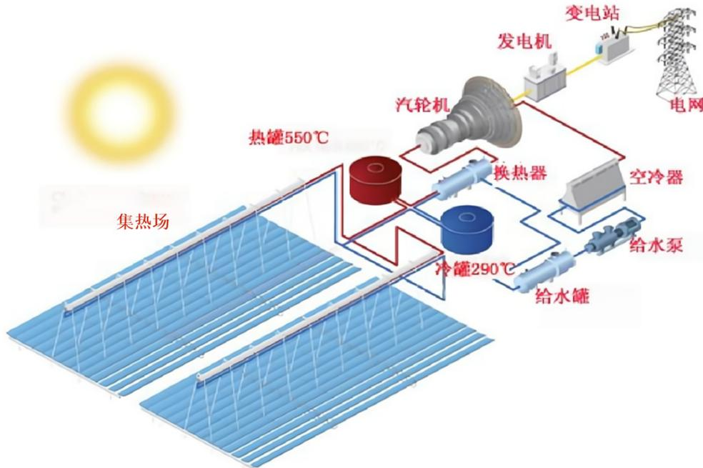
Diagram of a linear Fresnel CSP plant using a molten salt as the heat transfer medium (source: DCTC)
