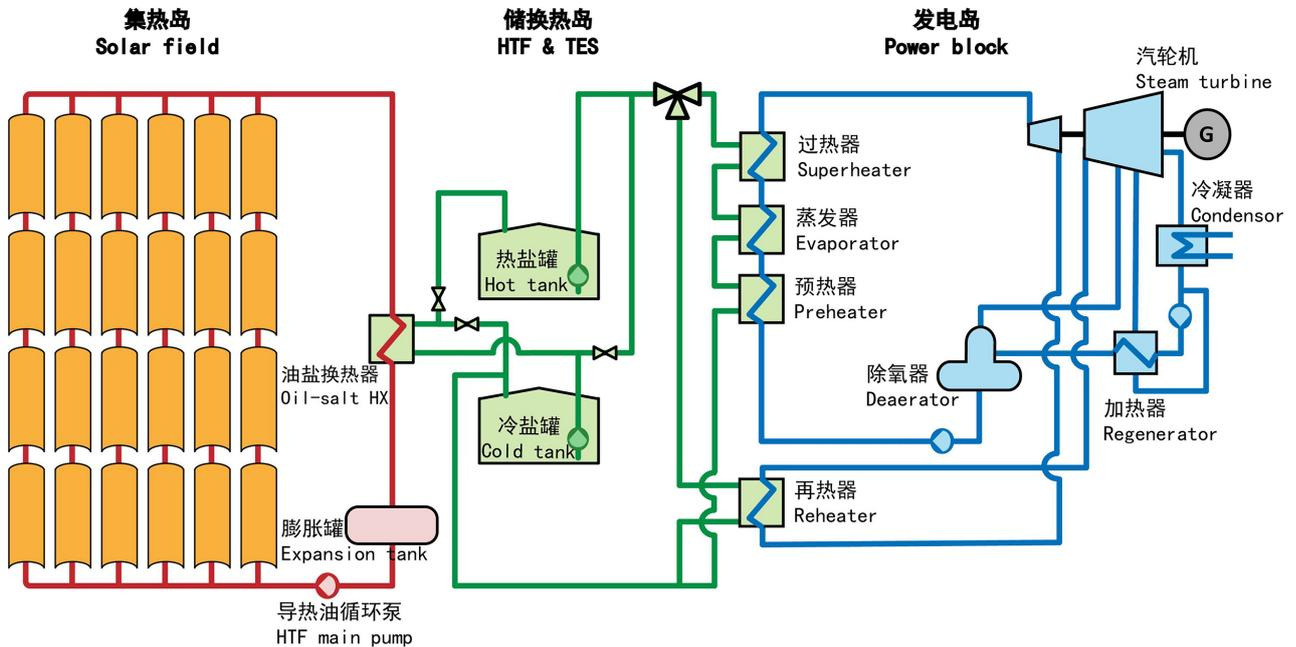
Diagram of a parabolic trough CSP plant (with decoupled processes) (source: ROYAL TECH CSP)
