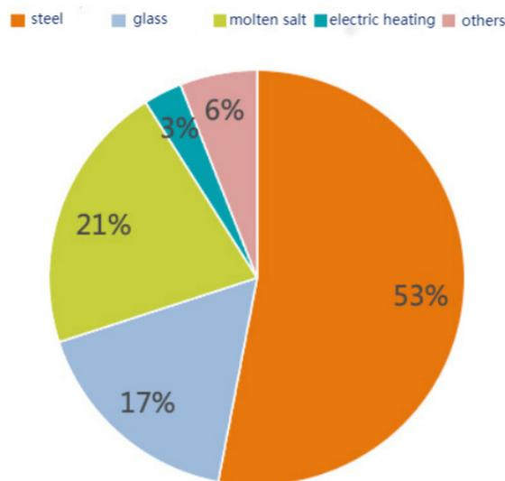
Figure: the cost proportion of raw materials in solar field, heat collection and thermal storage subsystems of Qinghai Supcon Delingha 50MW solar tower plant
