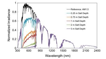
Fig. 6. Solar irradiance attenuation for different molten salt depths. This figure was produced using experimentally measured attenuation coefficients for a 60/40 wt.% sodium–potassium nitrate mixture at 350 °C in the wavelength range of 400–800 nm, the range where experimental measurements are possible.
