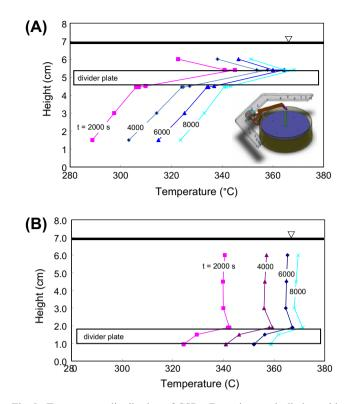
Fig. 8. Temperature distribution of CSPonD receiver optically heated by the 10.5 kW MIT CSP solar simulator; inset depicts stainless steel (type 316 L, 28 cm inner diameter  $\times$  8 cm high, 7 L solar salt capacity) test receiver. The movable divider plate (3.2 mm thick stainless steel disk with a 6.4 mm thick layer of rigid silica insulation board affixed to the underside) and is denoted by the shaded gray box located near the salt surface (A) and tank bottom (B) of the test receiver.
