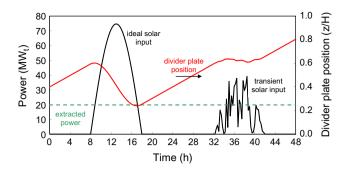
Fig. 3. Simplified divider plate position example for two day/night cycles: Ideal solar input (left) and transient, or cloudy, solar input (right) for a constant 20  $MW_t$  extraction system.
