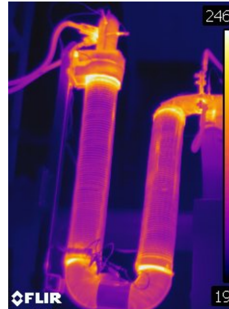
Impedance heating to 550 °C
