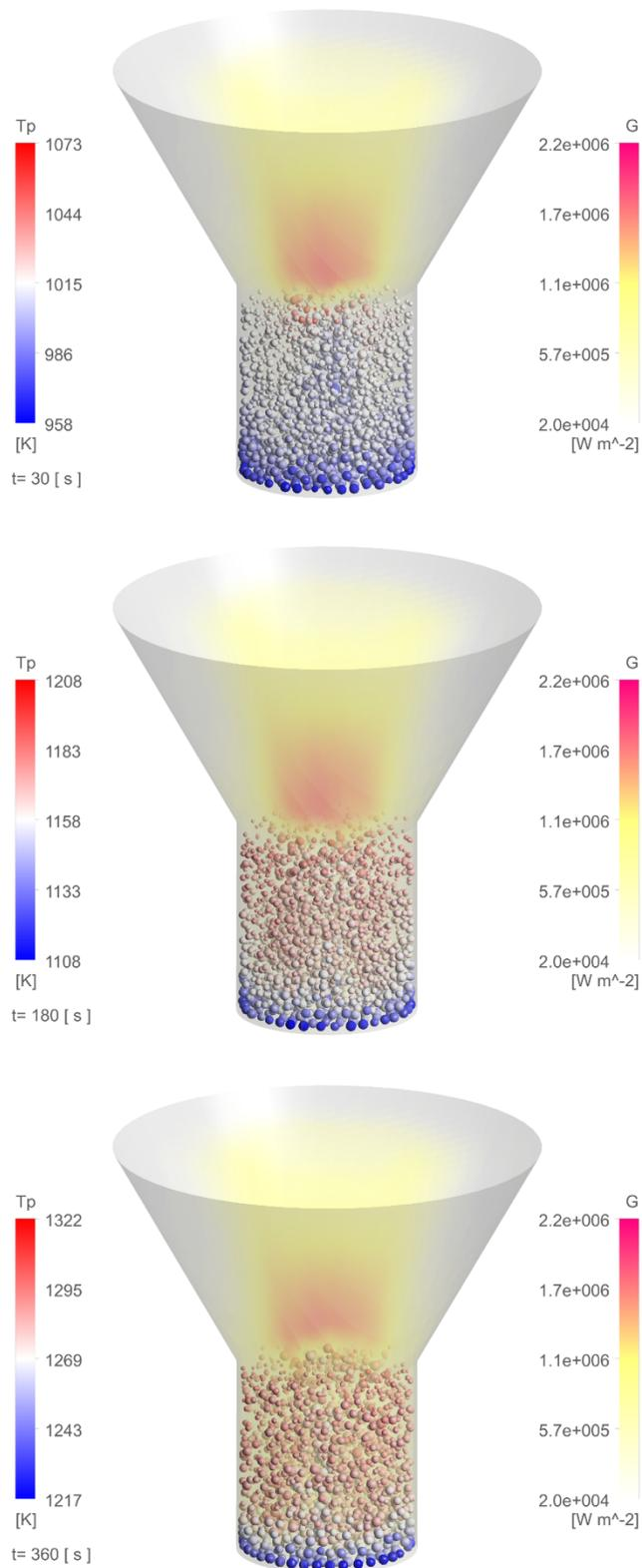
**FIGURE 2.** Three dimensional temperature distribution of the discrete phase particle along with the incident radiation at different instants.
