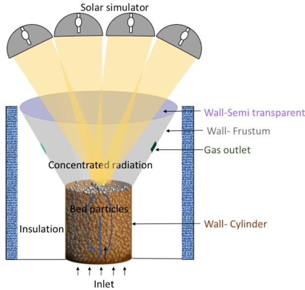
FIGURE 1. Schematic and computational geometry of the reactor
