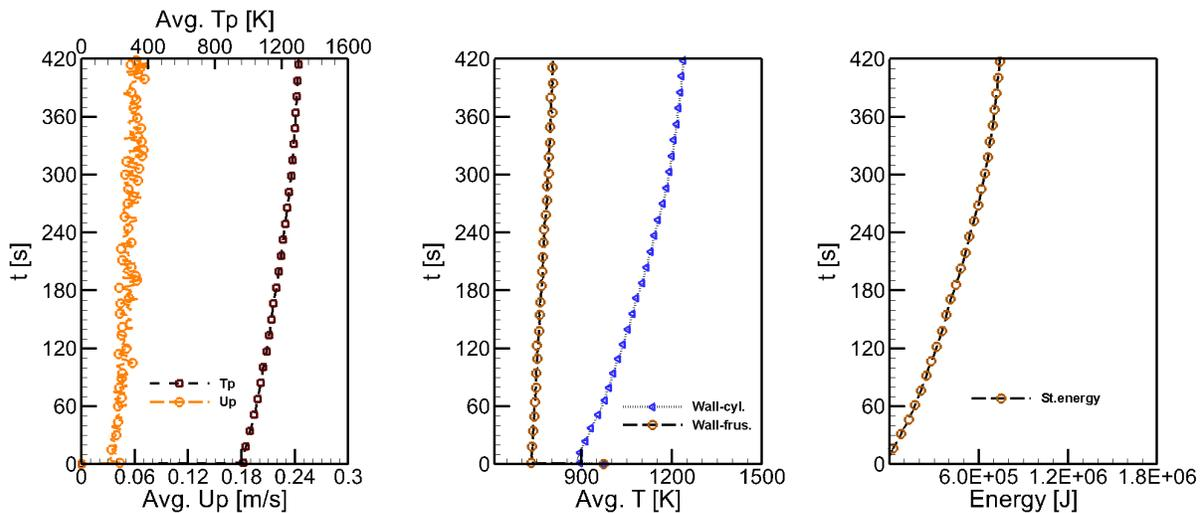
**FIGURE 5.** Average temperature and velocity of the particles as a function of time along with the average wall temperature and total energy stored in the bed.
