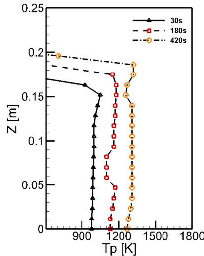
**FIGURE 3.** Instantaneous temperature distribution of the particle phase at the central axis.
