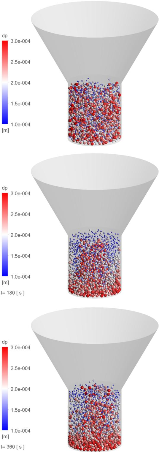
**FIGURE 4.** Particle size distribution at different instants, at 1, 180 and 360 s.
