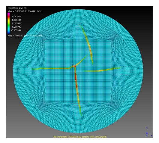
\* Analysis background is successively apply salt pressure load, temperature difference, remove temperature load, remove pressure and look at final, permanently deformed floor shape. The height of the ridges in the plot are approximately the same as the height of the ridges in the photo a couple of slides before
