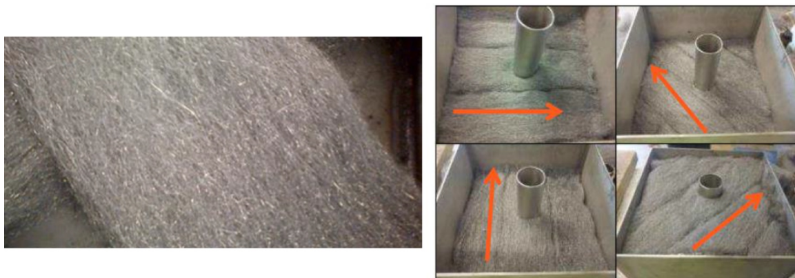
Fig. 2. Metal wool inserted in the storage tank.
