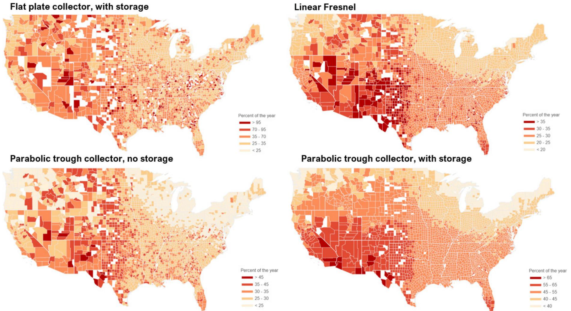
**Figure 14. County-level maps showing the percentage of the year when solar heat is fully meeting process heat demand using solar thermal technologies (FPCs, LF DSG, PTC with TES, and PTC without TES) sized to peak summer demand**
