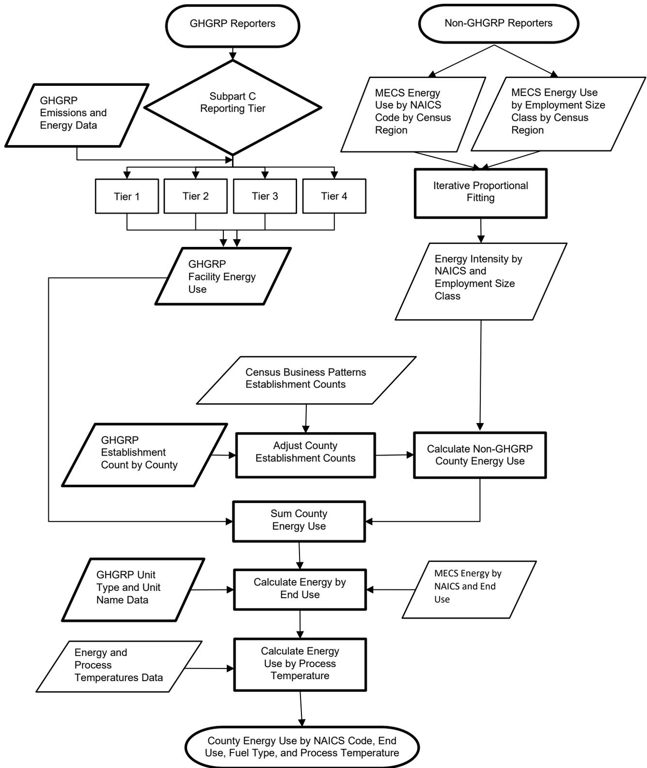
**Figure B-1. General process for estimating 2014 county-level industrial process heat demand**
