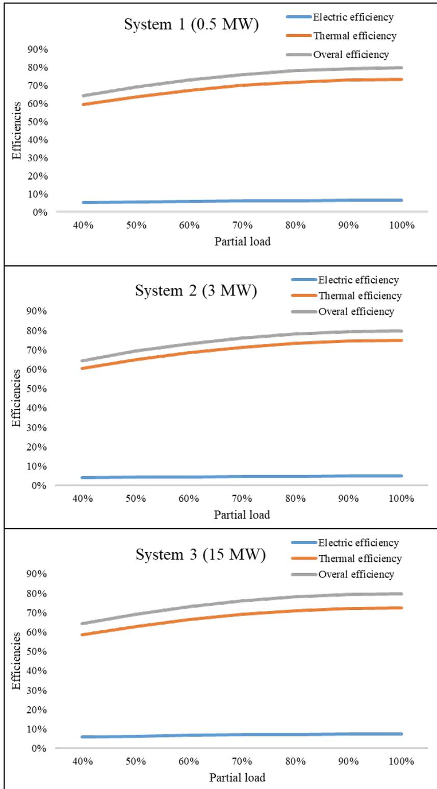
Figure A-3. Thermal, electric, and overall efficiencies of steam turbine CHP systems with different capacities
