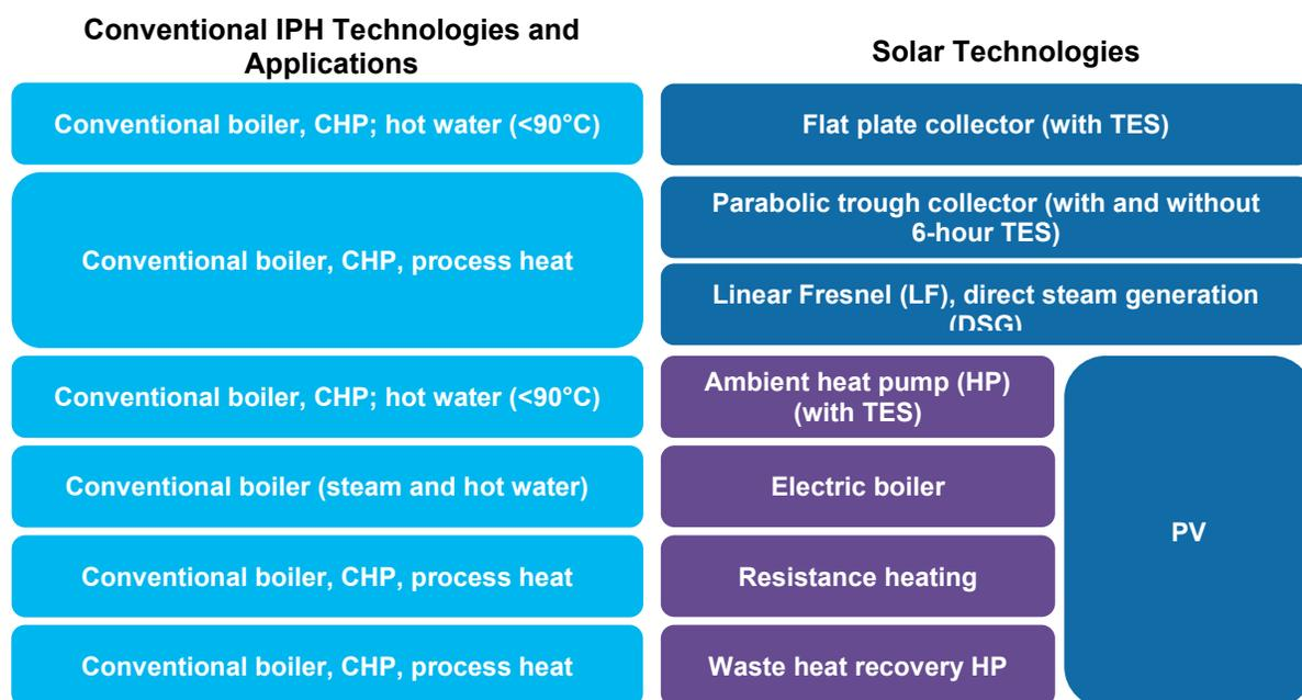
**Figure 1. Applications of industrial process heat matched to relevant solar technologies**
