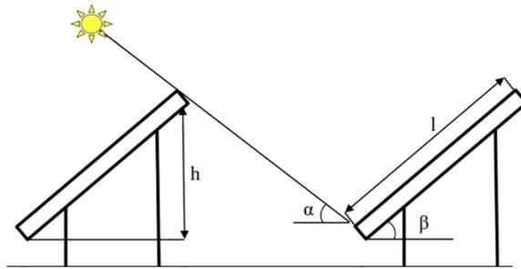
**Figure E-4. Ground coverage factor (GCF) and the PV panels relative to the sun**
