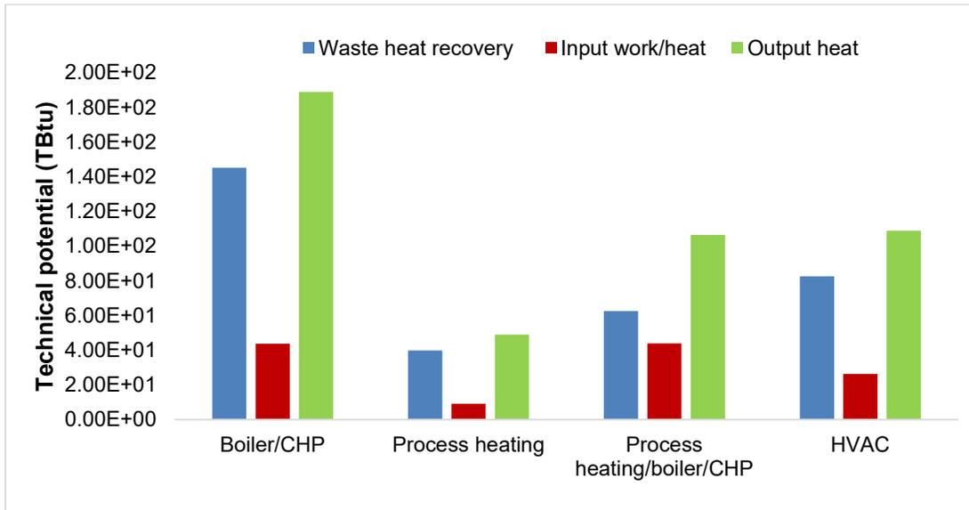
**Figure A-1. Technical potential of WHRHPs associated with different end uses**
