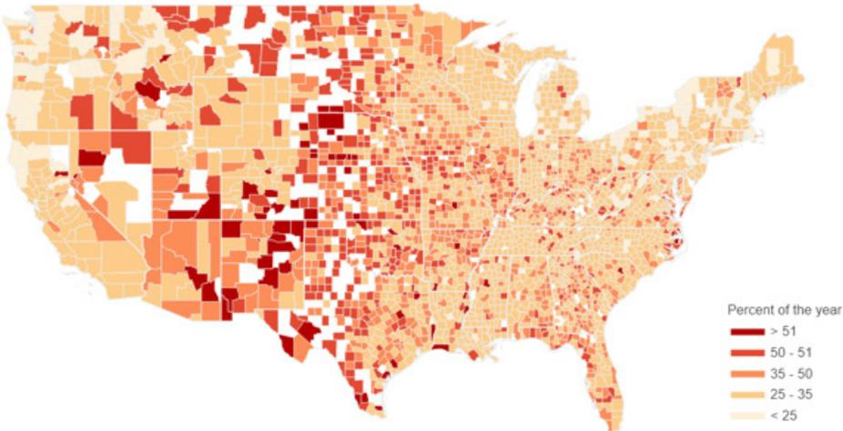
**Figure 15. County-level maps showing the percentage of the year when solar heat is fully meeting demand using PV-based electrotechnologies (E-boiler, resistance heating and WHRHPs) sized to peak summer demand**
