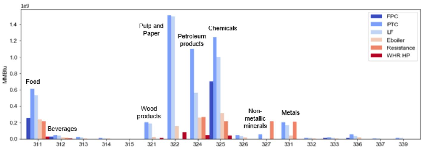
**Figure C-3. Process heat demands for each solar technology package by industrial subsector**
