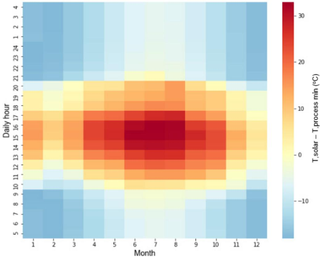
**Figure 27. Heat map of the difference between the minimum required process temperature in Bee County in Texas (36°C) and the temperature of hot water supplied by an FPC system**
