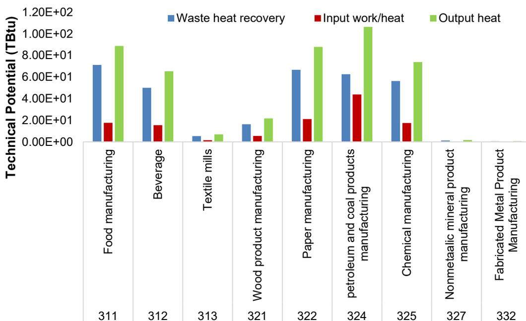
**Figure 6. Estimated technical potentials of using waste heat recovery heat pumps (WHRHPs)**
