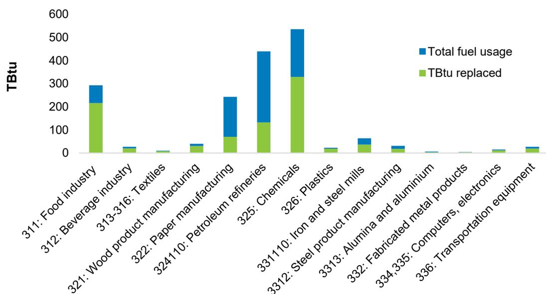
**Figure 5. Total fuel use of conventional boilers and technical potential of using electric boilers to replace conventional boilers**
