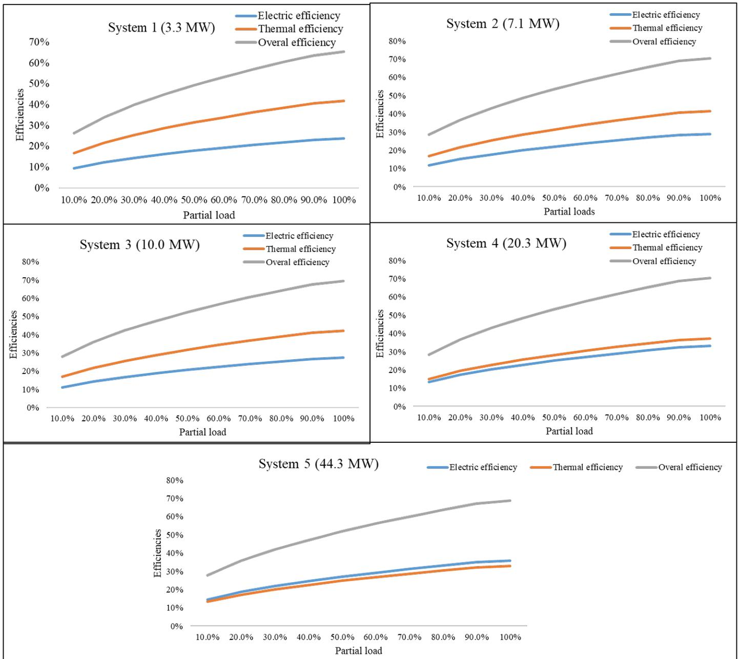
**Figure A-2. Thermal, electric, and overall efficiencies of combustion/gas turbine CHP systems with different capacities**
