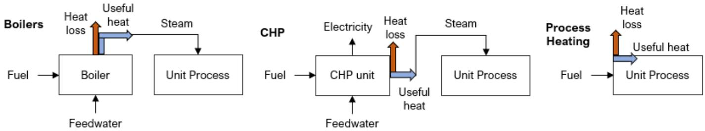
**Figure 9. Block diagrams of the three end-use categories for IPH**
