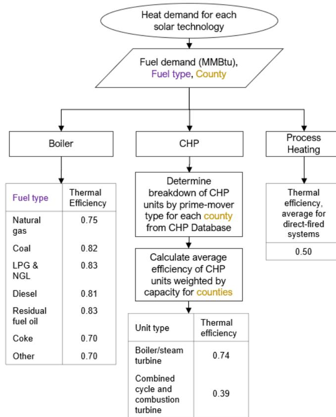
**Figure C-2. Flowchart for determining efficiencies of IPH end uses**
