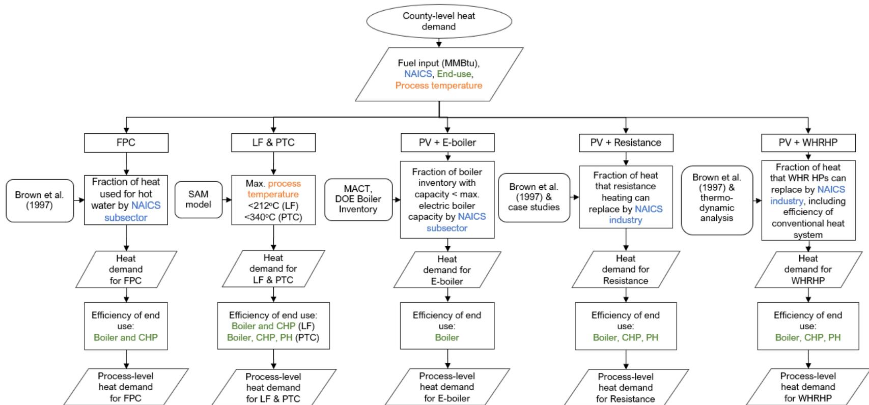
**Figure C-1. Flowchart for calculating process energy for each solar technology package**
