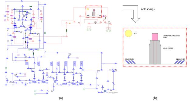
FIGURE 2. The PHOTON project: Solar thermal electric plant system configuration with highlighted solar thermal power tower (100 MWe case example – property of Acciona) [3].
