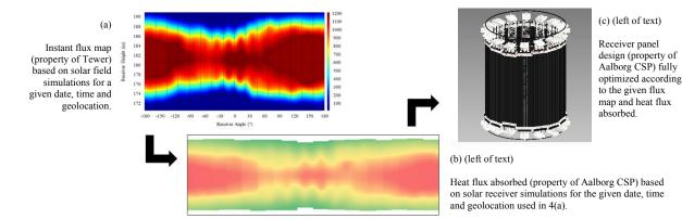
FIGURE 4. The PHOTON project: 100 MWe Asymmetric MSR design phase steps based on an incident flux map [12].
