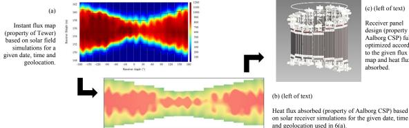
FIGURE 6. The PHOTON project: 50 MWe Asymmetric MSR design phase steps based on an incident flux map [12].
