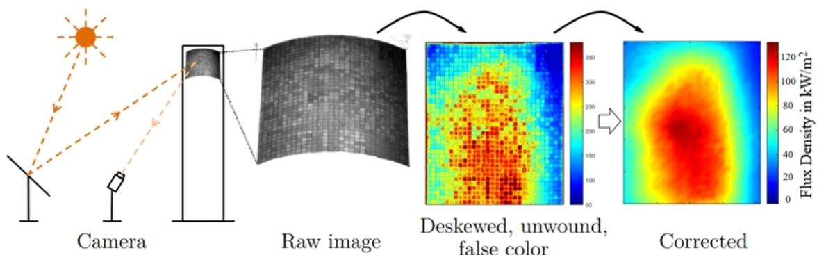
*A camera takes pictures of the surface of a solar receiver during solar operation. By applying various correction matrices and calibrating with a radiometer, the rectified raw image turns into an image of the solar flux density distribution in kW/m<sup>2</sup>.
