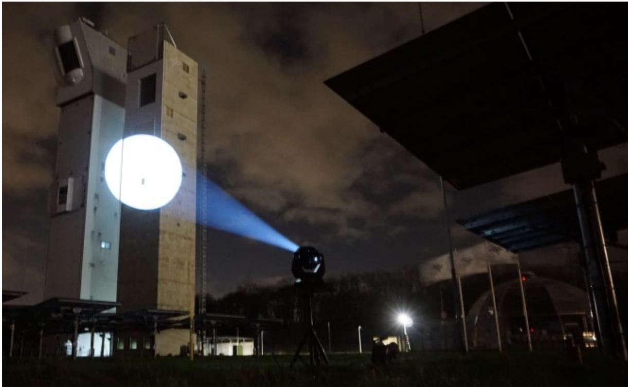
*With a patented scanning process, the reflection properties of the receiver surface are determined at night. This is necessary just once for the installation of the system. These data will later be used to correct the raw images. Image: DLR*
