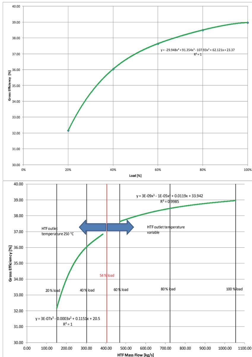
Figure 6-5: Impact of load and HTF inlet temperature on gross efficiency,  $\eta_{\text{gross}}^{\text{PB}}$ , for a thermal oil driven Rankine cycle. The upper figure shows the data plotted as a function of normalized thermal power,  $\dot{Q}^{\text{PB}}/\dot{Q}_0^{\text{PB}}$ , the lower figure as function of HTF mass flow,  $\dot{m}^{\text{PB}}$ .
