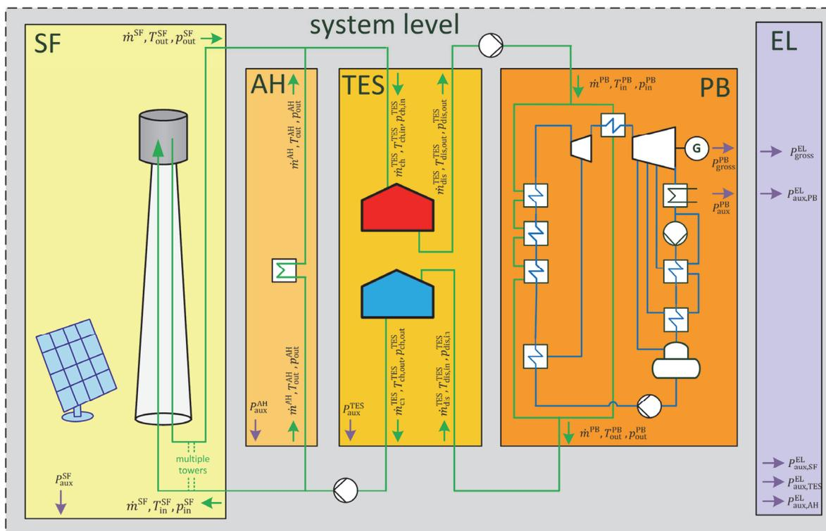
Figure 4-2: Sub-system schematic with main interface variables for a molten salt tower plant
