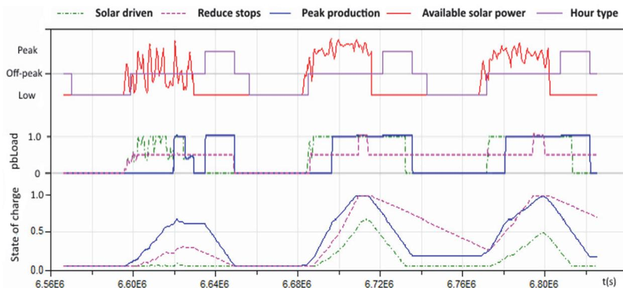
Figure 10-1: STE power plant operation with three different operation strategies. In this exemplary calculation the peak production strategy increases the energy revenues by 1.3 % while the reduced stops strategy reduces it by 14.5 % (taken from: Javier García-Barberena, Ioseba Erdocia: “Simulation and Comparison of Different Operational Strategies for Storage Utilization in Concentrated Solar Power Plants”, SolarPACES2015 conference, Cape Town, South Africa, 13.-15. October 2015).
