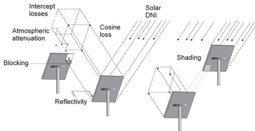
Figure 5-7: Illustration of optical losses in the heliostat field
