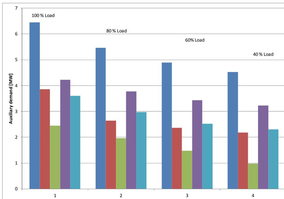
Figure 6-6:Auxiliary electrical consumption for different electrical load cases of a 50 MW power block equipped with ACC. The five bars refer to different designs of the same configuration.
