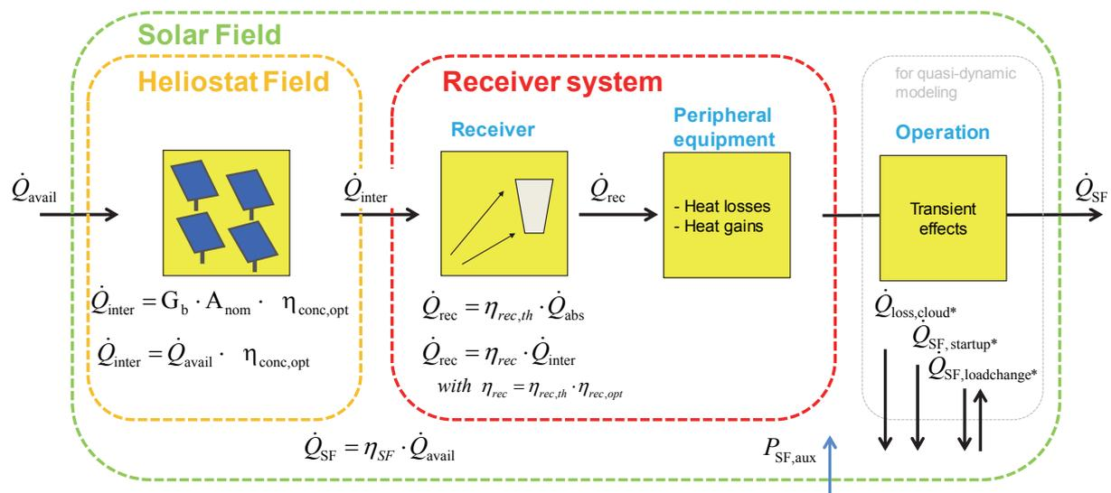
Figure 5-6: Illustration of sub-system solar field for solar towers and its parts
