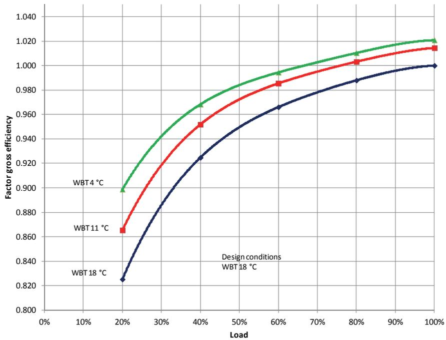
Figure 6-3: Impact of load,  $\dot{Q}^{PB}/\dot{Q}_0^{PB}$ , and wet bulb temperature on gross efficiency correction function  $f_1$  for a thermal oil driven Rankine cycle with wet cooling tower.
