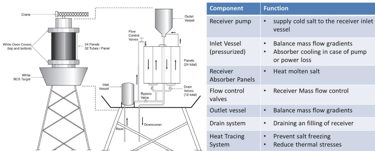
Figure 5-9: Components of a receiver system of a molten salt tower<sup>17</sup>
