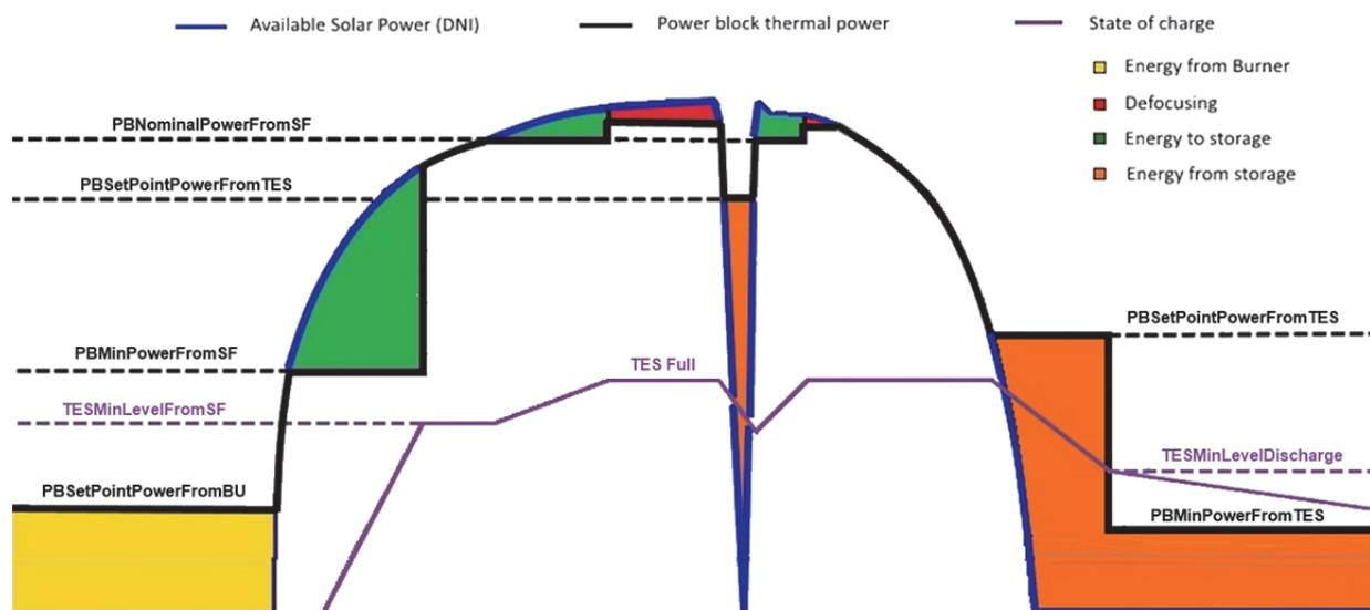
Figure 10-4: Conceptual behavior of the power block power (black, solid), storage state of charge (purple, solid) and available solar power (blue, solid) for a reference day according to the flexible operational strategy.
