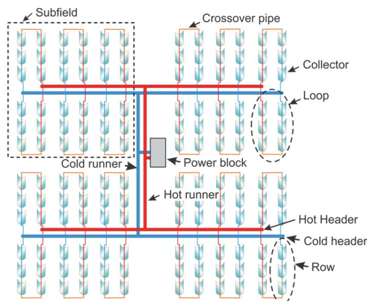
Figure 5-5: Typical layout of a parabolic trough STE plant and definition of the sections
