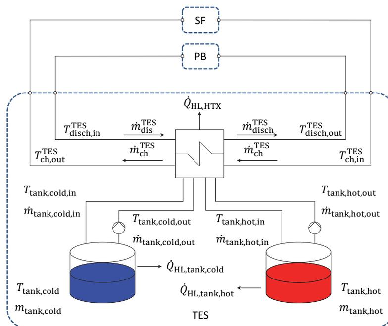
Figure 7-3 Scheme of a two-tank indirect molten salt storage system
