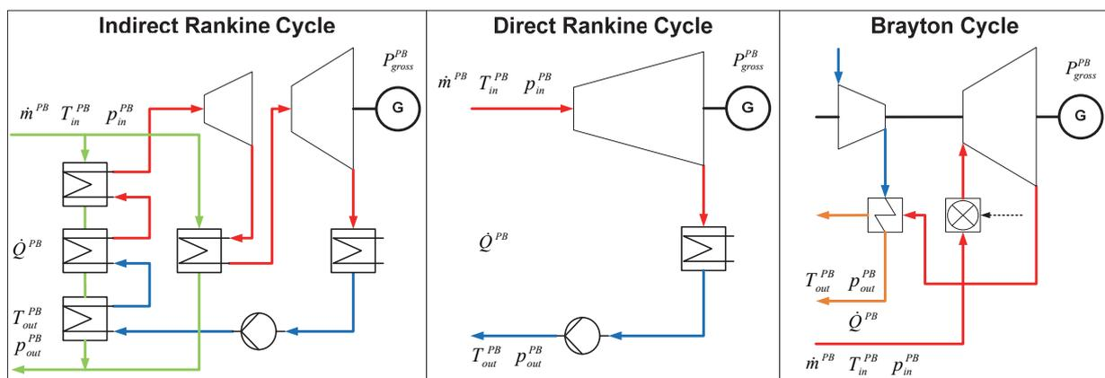
Figure 6-1: Sub-system boundaries for three types of power block configurations
