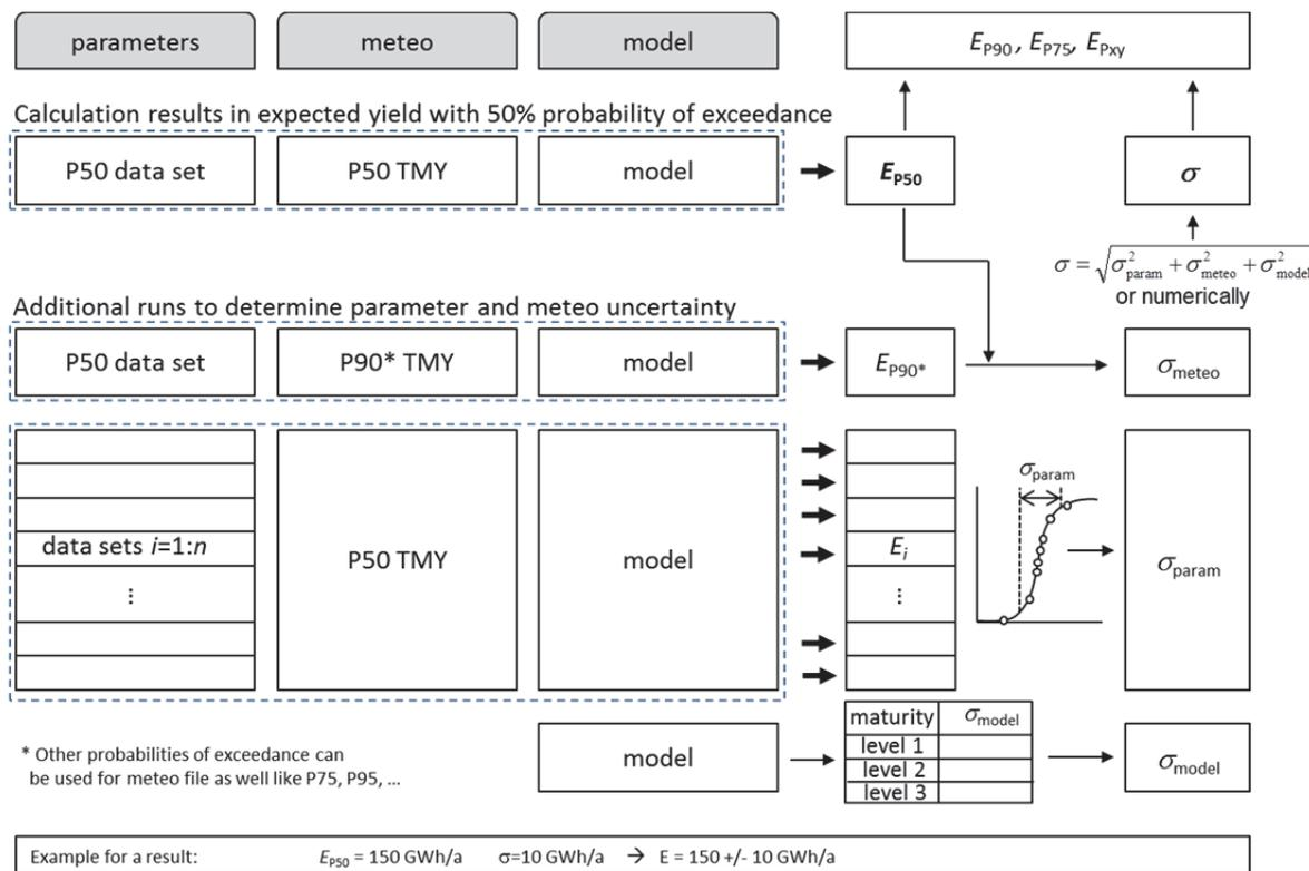
Figure 13-3: Structured approach to determining overall uncertainty based on the three categories parameter uncertainty, model uncertainty, and uncertainty of the meteorological input data.
