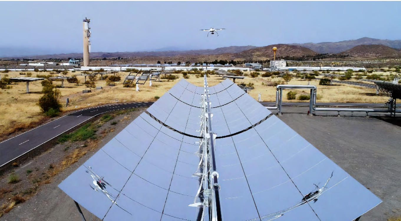
Airborne quality control of a parabolic trough. Photograph taken at the Plataforma Solar de Almería (PSA). The Spanish research centre CIEMAT is the owner and operator of the PSA.
