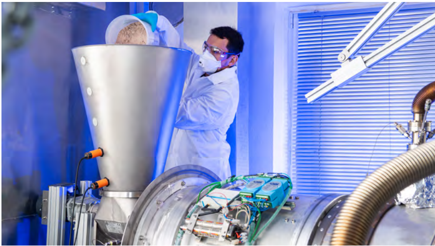
At DLR's solar simulator in Cologne researchers successfully tested the solar-powered calcination of raw cement powder as a step in cement production. Credit: DLR
