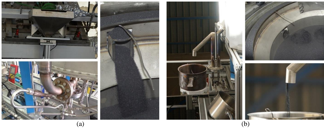
FIGURE 2. Continuous particles supply (a) and removal (b).
